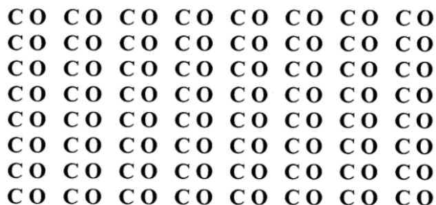
Figure 2. A two-dimensional representation of a perfect CO crystal.
