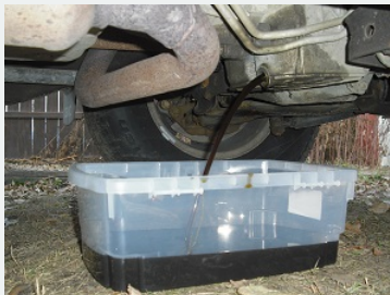
Figure 16.6.5: Oil being drained from a car
