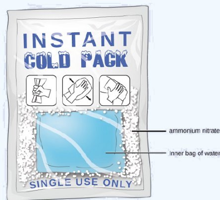
Figure 13.3.1.5: An instant cold pack consists of a bag containing solid ammonium nitrate and a second bag of water. When the bag of water is broken, the pack becomes cold because the dissolution of ammonium nitrate is an endothermic process that removes thermal energy from the water. The cold pack then removes thermal energy from your body.
