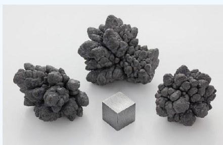
Electrolytically refined pure (99.989 %) superficially oxidized lead nodules and a high purity (99.989 %) 1 cm 3 lead cube for comparison. Figure used with permission from Wikipedia.
