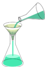
Figure 11.2.1: When a colored solution is passed through a filter, the entire solution, both solute and solvent, pass through unchanged.
