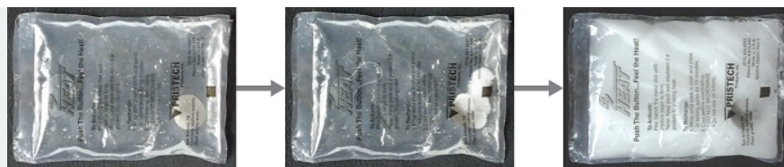
Figure 13.3.1.5: Chemical hand warmers produce heat that warms your hand on a cold day. In this one, you can see the metal disc that initiates the exothermic precipitation reaction. (credit: modification of work by Science Buddies TV/YouTube)
