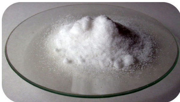
Figure 11.2.5: Calcium nitrate is a typical ionic compound. In an aqueous solution, it dissociates into calcium ions and nitrate ions.
