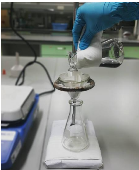
Figure 2.4.4: Filtration for the separation of solids from a hot solution. (CC BY-SA 4.0; Suman6395).
