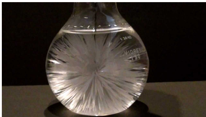
Figure 2.1.4: The Crystallization of Sodium Acetate from a Concentrated Solution of Sodium Acetate in Water. The addition of a small “seed” crystal (a) causes the compound to form white crystals, which grow and eventually occupy most of the flask. Video can be found here: www.youtube.com/watch?v=BLq5NibwV5g
