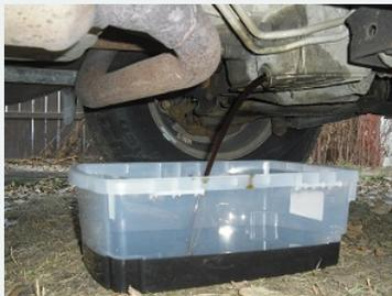
Figure 16.6.5: Oil being drained from a car
