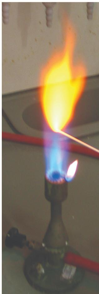
Figure 11.2.4: Dipping a wire into a solution of a sodium salt and then heating the wire causes emission of a bright yellow light, characteristic of sodium.
