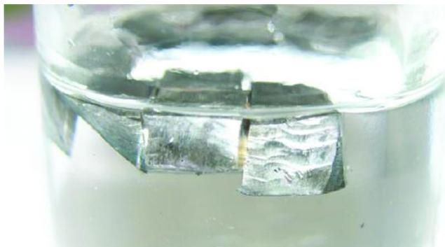
Figure 11.2.2: Lithium floats in paraffin oil because its density is less than the density of paraffin oil.
