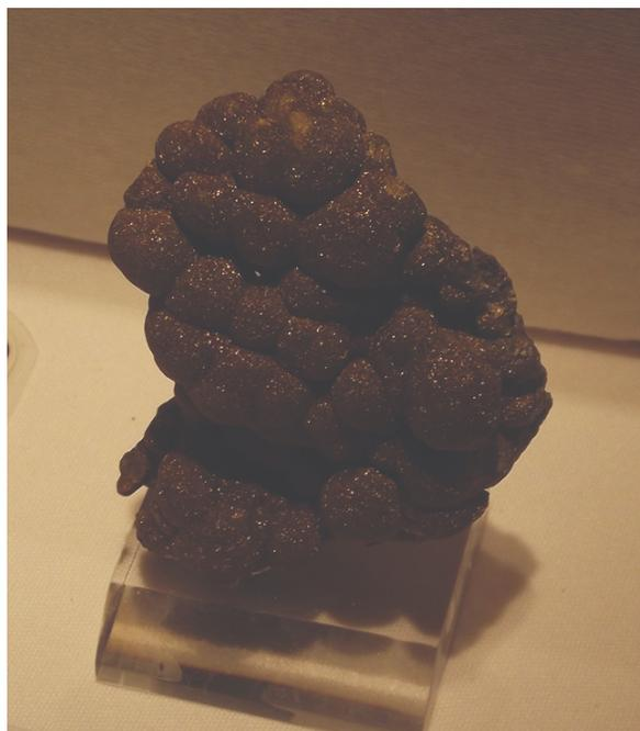
Figure 6.2.7: Blister copper is obtained during the conversion of copper-containing ore into pure copper. (credit: “Tortie tude”/Wikimedia Commons)
