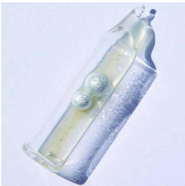
Figure 11.2.3: To prevent contact with air and water, potassium for laboratory use comes as sticks or beads stored under kerosene or mineral oil, or in sealed containers. (credit: <http://images-of-elements.com/potassium.php>)
