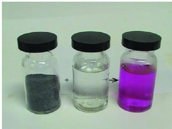
Figure 11.2.5: From left to right: Mg(s), warm water at pH 7, and the resulting solution with a pH greater than 7, as indicated by the pink color of the phenolphthalein indicator. (credit: modification of work by Sahar Atwa)
