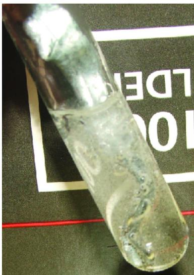
Figure 11.2.6: Zinc is an active metal. It dissolves in hydrochloric acid, forming a solution of colorless  $\text{Zn}^{2+}$  ions,  $\text{Cl}^-$  ions, and hydrogen gas.
