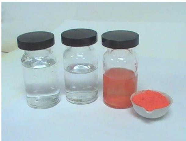
Figure 11.12.2: Solid  $\text{HgI}_2$  forms when solutions of  $\text{KI}$  and  $\text{Hg(NO}_3)_2$  are mixed. (credit: Sahar Atwa)
