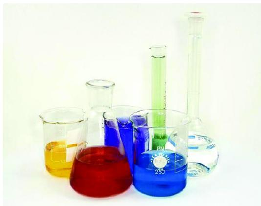
Figure 11.4.4: Laboratory glassware, such as Pyrex and Kimax, is made of borosilicate glass because it does not break when heated. The inclusion of borates in the glass helps to mediate the effects of thermal expansion and contraction. This reduces the likelihood of thermal shock, which causes silicate glass to crack upon rapid heating or cooling. (credit: "Tweenk"/Wikimedia Commons)
