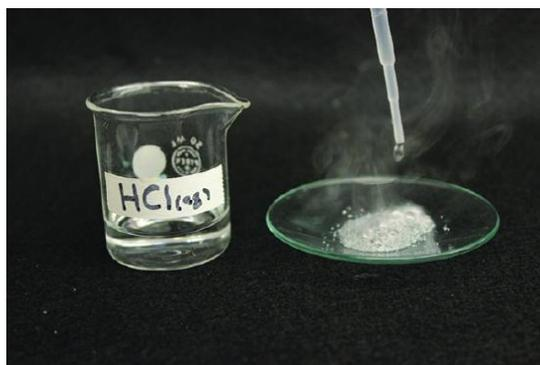
Figure 11.6.2: The reaction of iron with an acid produces hydrogen. Here, iron reacts with hydrochloric acid.(credit: Mark Ott)
