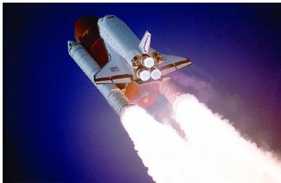
Figure 11.6.3: Before the fleet's retirement in 2011, liquid hydrogen and liquid oxygen were used in the three main engines of a space shuttle. Two compartments in the large tank held these liquids until the shuttle was launched.(credit: "reynermedia"/Flickr)
