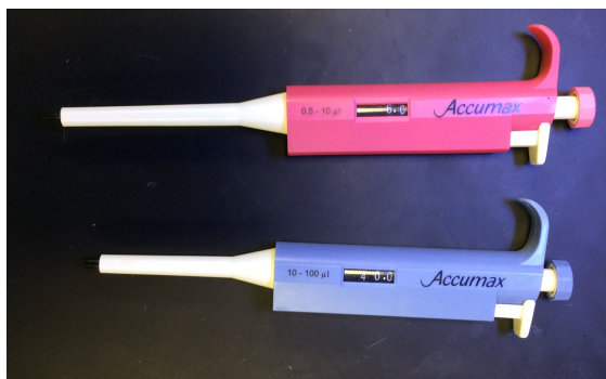
Figure 2.4.4 : A set of two digital micropipets. The pipet on the top delivers volumes between 0.5 mL and 10 \mu L and the pipet on the bottom delivers volumes between 10 mL and 100 \mu L.
