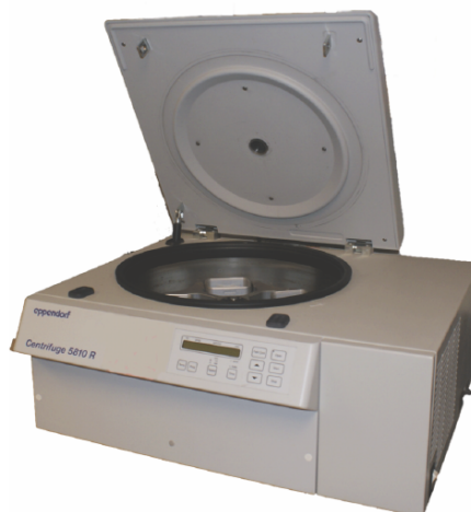
Figure 7.6.3 . Bench-top centrifuge capable of reaching speeds up to 14000 rpm and centrifugal forces of 20800 \times g . This particular centrifuge is refrigerated, allowing samples to be cooled to temperatures as low as -4^{\circ}\text{C} .
