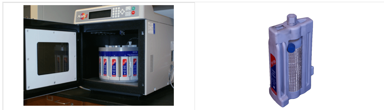
Figure 7.3.7 . Microwave digestion unit: on the left is a view of the unit's interior showing the carousel that holds the digestion vessels; on the right is a close-up of a Teflon digestion vessel, which is encased in a thermal sleeve. The pressure relief valve, which is part of the vessel's blue cap, contains a membrane that ruptures if the internal pressure becomes too high.
