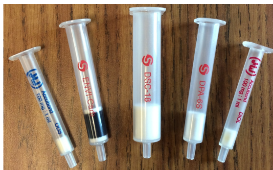
Figure 7.6.10 . Selection of solid phase extraction cartridges for liquid samples. The solid adsorbent is the white or black material in each cartridge. From left-to-right, the adsorbent materials are octadecylsilane, carbon, octadecylsilane, polyamide resin, and diol; see Table 7.6.5 for additional details. The size of the cartridges dictates the volume of sample used; from left-to-right, these cartridges use samples of 1 mL, 3 mL, 6 mL, 3 mL, and 1 mL.
