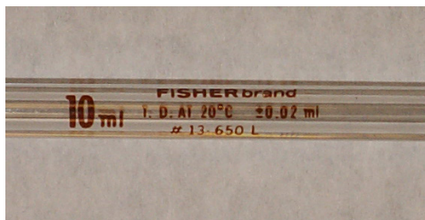
Figure 4.2.1 : Close-up of a 10-mL volumetric pipet showing that it has a tolerance of \pm 0.02 mL at 20 °C.
