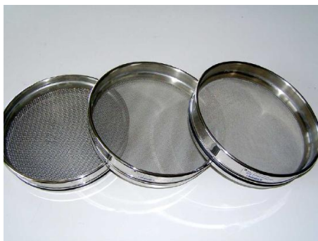
Figure 8.4.1 . Three sieves with, from left to right, mesh sizes of 1700 \mu\text{m} , 500 \mu\text{m} , and 250 \mu\text{m} . Source: BMK ( commons.wikimedia.com ).
