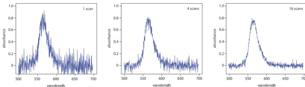
**Figure 10.3.5** . Effect of signal averaging on a spectrum's signal-to-noise ratio. From top to bottom: spectrum for a single scan; average spectrum after four scans; and average spectrum after adding 16 scans.
