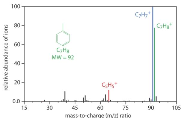
Figure 12.4.13 . Mass spectrum for toluene highlighting the molecular ion in green ( $m/z=92$ ), and two fragment ions in blue ( $m/z=91$ ) and in red ( $m/z=65$ ). A mass spectrum provides both quantitative and qualitative information: the height of any peak is proportional to the amount of toluene in the mass spectrometer and the fragmentation pattern is unique to toluene.
