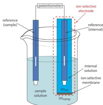
Figure 11.2.8 . Schematic diagram that shows a typical potentiometric cell with an **ion-selective electrode**. The ion-selective electrode's membrane separates the sample, which contains the analyte at an activity of  $(a_A)_{\text{somp}}$ , from an internal solution that contains the analyte with an activity of  $(a_A)_{\text{int}}$ .
