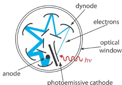
**Figure 10.1.14** . Schematic of a photomultiplier. A **photon** strikes the photoemissive cathode producing **electrons**, which accelerate toward a positively charged dynode. Collision of these electrons with the dynode generates additional electrons, which accelerate toward the next dynode. A total of  $10^6$ – $10^7$  electrons per photon eventually reach the anode, generating an electrical current.
