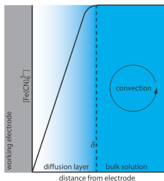
Figure 11.4.8 . Concentration gradient for  $\text{Fe}(\text{CN})_6^{3-}$  when stirring the solution. Diffusion is the only significant form of mass transport close to the electrode's surface. At distances greater than  $\delta$ , convection is the only significant form of mass transport, maintaining a homogeneous solution in which the concentration of  $\text{Fe}(\text{CN})_6^{3-}$  at  $\delta$  is the same as its concentration in bulk solution.
