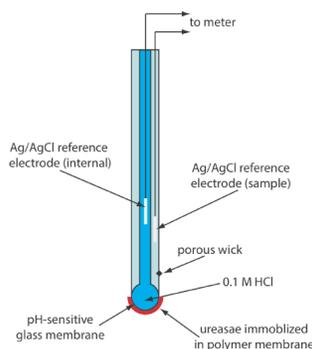
**Figure 11.2.15** . Schematic diagram of an enzyme-based potentiometric biosensor for urea in which urease is immobilized in a polymer membrane coated onto the pH-sensitive glass membrane of a pH electrode.
