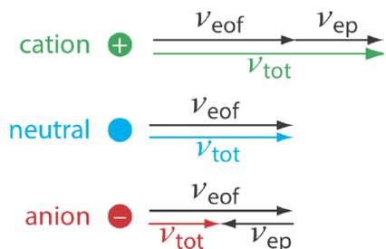
Figure 12.7.3 . Visual explanation for the general elution order in capillary electrophoresis. Each species has the same electroosmotic flow,  $\nu_{eof}$ . Cations elute first because they have a positive electrophoretic velocity,  $\nu_{ep}$ . Anions elute last because their negative electrophoretic velocity partially offsets the electroosmotic flow velocity. Neutrals elute with a velocity equal to the electroosmotic flow.
