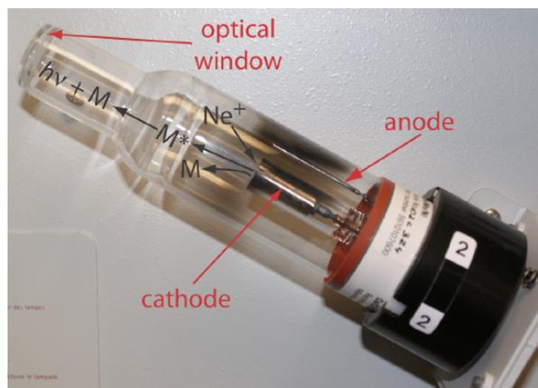
**Figure 10.4.5** . Photo of a typical multi-elemental hollow cathode lamp. The cathode in this lamp is fashioned from an alloy of Co, Cr, Cu, Fe, Mn, and Ni, and is surrounded by a glass shield that isolates it from the anode. The lamp is filled with Ne gas. Also shown is the process that leads to atomic emission. Note the black deposit of sputtered metal on the outer wall of the hollow cathode lamp. See the text for additional details.
