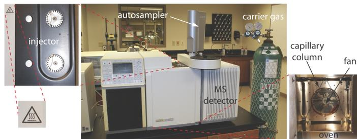
**Figure 12.4.1** . Example of a typical gas chromatograph with insets showing the heated injection ports—note the symbol indicating that it is hot—and the oven that houses the column. This particular instrument is equipped with an autosampler for injecting samples, a capillary column, and a mass spectrometer (MS) as the detector. Note that the carrier gas is supplied by a tank of compressed gas.
