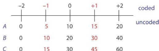
Figure 14.1.14 . The relationship between the coded factor levels and the uncoded factor levels for Example 14.1.3 . The numbers in red are the values defined in the  $2^3$  factorial design.
