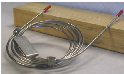
**Figure 12.4.2** . Typical example of a packed column for gas chromatography. This column is made from stainless steel and is 2 m long with an internal diameter of 3.2 mm. The packing material in this column has a particle diameter of 149–177 μm. To put this in perspective, beach sand has a typical diameter of 700 μm and the diameter of fine grained sand is 250 μm.
