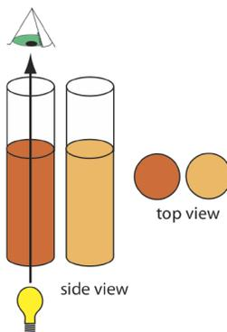
**Figure 10.1.9**. Nessler's original method for comparing the color of two solutions. Natural light passes upwards through the samples and standards and the analyst views the solutions by looking down toward the light source. The top view, shown on the right, is what the analyst sees. To determine the analyte's concentration, the analyst exchanges standards until the two colors match.
