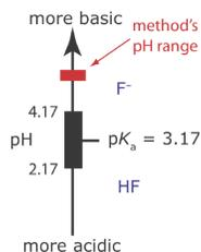
**Figure 11.2.17**. Ladder diagram for HF/ $F^-$ . Maintaining a pH greater than 4.2 ensures that the only significant form of fluoride is  $F^-$ .
