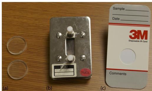
**Figure 10.3.8** . Three examples of IR sample cells: (a) NaCl salts plates; (b) fixed pathlength (0.5 mm) sample cell with NaCl windows; (c) disposable card with a polyethylene window that is IR transparent with the exception of strong absorption bands at  $2918\text{ cm}^{-1}$  and  $2849\text{ cm}^{-1}$ .
