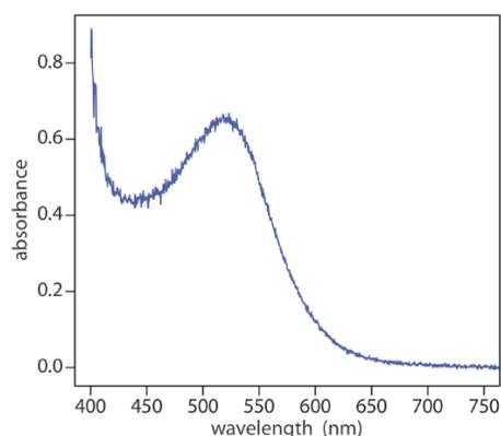
**Figure 10.1.5** . Visible absorbance spectrum for cranberry juice. The anthocyanin dyes in cranberry juice absorb visible light with blue, green, and yellow wavelengths (see Figure 10.1.3 ). As a result, the juice appears red.
