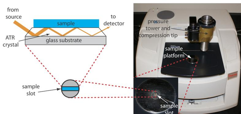
**Figure 10.3.9** . FT-IR spectrometer equipped with a diamond ATR sample cell. The inserts show a close-up photo of the sample platform, a sketch of the ATR's sample slot, and a schematic showing how the source's radiation interacts with the sample. The pressure tower is used to ensure proper contact of a solid sample with the ATR crystal.
