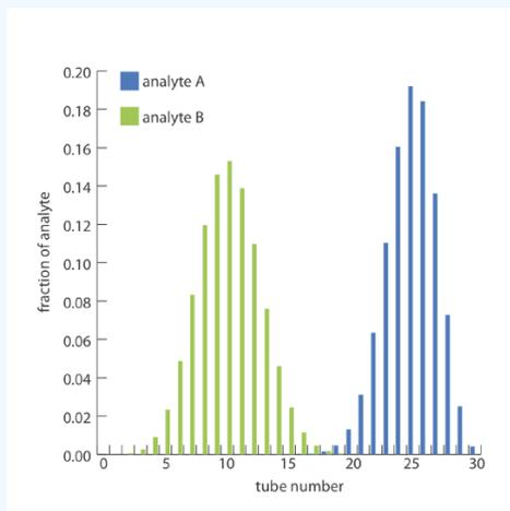
Figure 16.16.3. Progress of a countercurrent extraction for the separation of analyte A and B showing the fraction of analyte in each tube after 30 steps. The distribution ratio,  $D$ , is 5.0 for analyte A and 0.5 for analyte B. The volumes of the two phases are identical.
