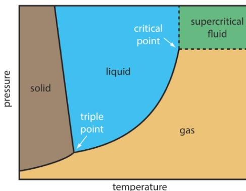
Figure 12.6.4 . Phase diagram showing the combinations of temperature and pressure for which a compound is in its **solid state**, its **liquid state**, and its **gas state**. For pressures and temperatures above the critical point, the compound is a **supercritical fluid** with properties intermediate between a gas and a liquid. Click [here](#) to see an interesting video demonstration of supercritical fluids from Nottingham Science City at the University of Nottingham.
