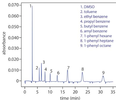
**Figure 12.7.10** . Capillary electrochromatographic separation of a mixture of hydrocarbons in DMSO. The column contains a porous polymer of butyl methacrylate and lauryl acrylate (25%:75% mol:mol) with butane dioldacrylate as a crosslinker. Data provided by Zoe LaPier and Michelle Bushey, Department of Chemistry, Trinity University.
