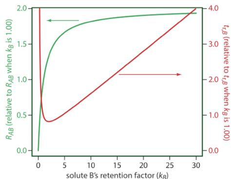
Figure 12.3.1. Effect of  $k_B$  on the resolution for a pair of solutes,  $R_{AB}$ , and the retention time for the later eluting solute,  $t_{r,B}$ . The y-axes display the resolution and retention time relative to their respective values when  $k_B$  is 1.00.
