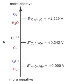
Figure 11.3.2 . Ladder diagram for an aqueous solution of  $\text{Cu}^{2+}$  showing steps for the reductions of  $\text{O}_2$  to  $\text{H}_2\text{O}$ , of  $\text{Cu}^{2+}$  to  $\text{Cu}$ , and of  $\text{H}_3\text{O}^+$  to  $\text{H}_2$ . For each step, the oxidized species is in blue and the reduced species is in red
