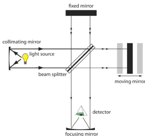
Figure 10.1.13 . Schematic diagram of an interferometers.
