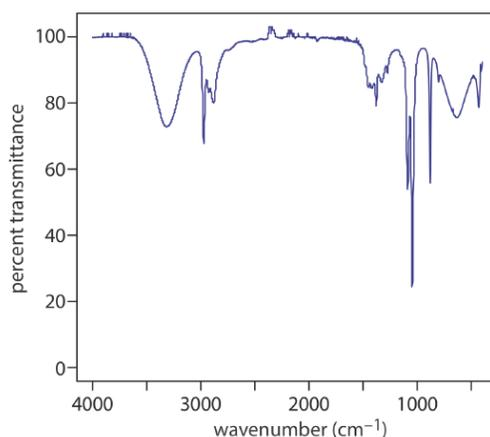
Figure 10.2.2 . Infrared spectrum of ethanol.
