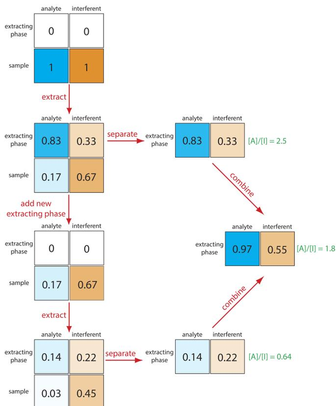
Figure 12.1.1 . Progress of a traditional liquid–liquid extraction using two identical extractions of a single sample using fresh portions of the extractant. The numbers give the fraction of **analyte** and **interferent** in each phase assuming equal volumes of sample and extractant and distribution ratios of 5 and 0.5 for the **analyte** and the **interferent**, respectively. The opacity of the colors equals the fraction of **analyte** and **interferent** present.
