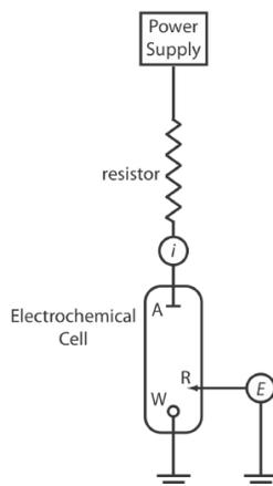
Figure 11.1.4 . Schematic diagram of a galvanostat: A is the auxiliary electrode; W is the working electrode; R is an optional reference electrode,  $E$  is a high-impedance potentiometer, and  $i$  is an ammeter. The working electrode and the optional reference electrode are connected to a ground.
