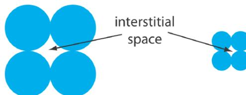
Figure 12.5.3 . The packing of smaller particles creates smaller interstitial spaces than the packing of larger particles. Although reducing particle size by 2 $\times$  increases efficiency by a factor of 1.4, it also produces a 4-fold increase in back pressure.
