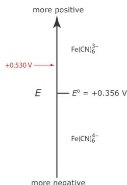
Figure 11.4.5 . Ladder diagram for the  $\text{Fe}(\text{CN})_6^{3-}/\text{Fe}(\text{CN})_6^{4-}$  redox half-reaction.
