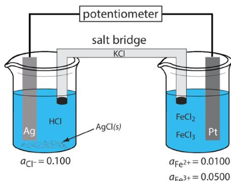
Figure 11.2.2 . Potentiometric electrochemical cell for Example 11.2.1 .
