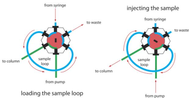
**Figure 12.5.8** . Schematic diagram of a manual loop injector. In the load position the flow of mobile phase from the pump to the column (shown in green) is isolated from the sample loop, which is filled using a syringe (shown in blue). Rotating the inner valve (shown in red) to the inject position directs the mobile phase through the sample loop and onto the column.
