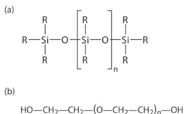
Figure 12.4.5 . General structures of common stationary phases: (a) substituted polysiloxane; (b) polyethylene glycol.
