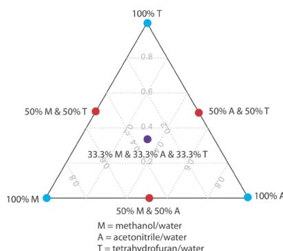
**Figure 12.5.4** . Solvent triangle for optimizing a reversed-phase HPLC separation. The three blue circles show mobile phases consisting of an organic solvent and water. The three red circles are binary mobile phases created by combining equal volumes of the pure mobile phases. The ternary mobile phase shown by the purple circle contains all three of the pure mobile phases.
