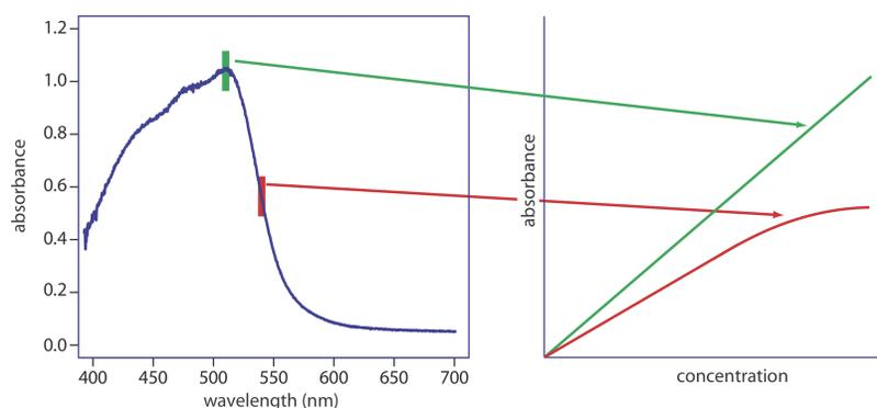
**Figure 10.2.10** . Effect of wavelength selection on the linearity of a Beer's law plot. Another reason for measuring absorbance at the top of an absorbance peak is that it provides for a more sensitive analysis. Note that the **green** Beer's law plot has a steeper slope—and, therefore, a greater sensitivity—than the **red** Beer's law plot. A Beer's law plot, of course, is equivalent to a calibration curve.
