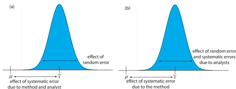
**Figure 14.3.1** . Partitioning of random errors, systematic errors due to the analyst, and systematic errors due to the method for (a) replicate analyses performed by a single analyst and (b) single determinations performed by several analysts.
