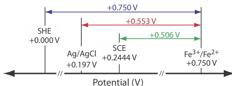
Figure 11.2.7 . Relationship between the potential of an  $\text{Fe}^{3+}/\text{Fe}^{2+}$  half-cell relative to the reference electrodes in Example 11.2.4 . The potential relative to a standard hydrogen electrode is shown in blue, the potential relative to a saturated silver/silver chloride electrode is shown in red, and the potential relative to a saturated calomel electrode is shown in green.
