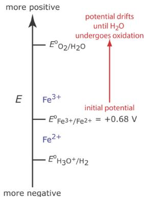
Figure 11.3.5 . Ladder diagram for the constant-current coulometric analysis of  $\text{Fe}^{2+}$ . The red arrow and text shows how the potential drifts to more positive values, decreasing the current efficiency.
