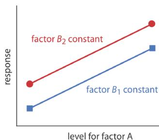
Figure 14.1.6 . Factor effect plot for two independent factors. Note that the two lines are parallel, indicating that the level for factor  $B$  does not influence how factor  $A$ 's level affects the response.
