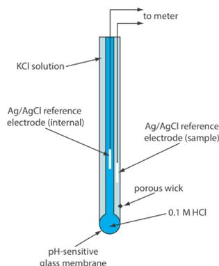
**Figure 11.2.10.** Schematic diagram showing a combination glass electrode for measuring pH. The indicator electrode consists of a pH-sensitive glass membrane and an internal Ag/AgCl reference electrode in a solution of 0.1 M HCl. The sample's reference electrode is a Ag/AgCl electrode in a solution of KCl (which may be saturated with KCl or contain a fixed concentration of KCl). A porous wick serves as a salt bridge between the sample and its reference electrode.
