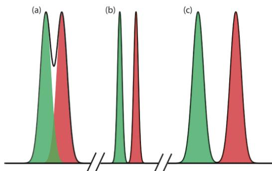
Figure 12.2.7 . Two method for improving chromatographic resolution: (a) original chromatogram; (b) chromatogram after decreasing  $w_A$  and  $w_B$  by 4×; and (c) chromatogram after increasing  $\Delta t_r$  by 2×.
