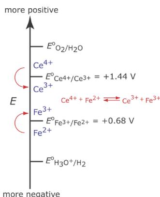
Figure 11.3.6 . Ladder diagram for the constant-current coulometric analysis of  $\text{Fe}^{2+}$  in the presence of a  $\text{Ce}^{3+}$  mediator. As the potential drifts to more positive values, we eventually reach a potential where  $\text{Ce}^{3+}$  undergoes oxidation. Because  $\text{Ce}^{4+}$ , the product of the oxidation of  $\text{Ce}^{3+}$ , reacts with  $\text{Fe}^{2+}$ , we maintain current efficiency.
