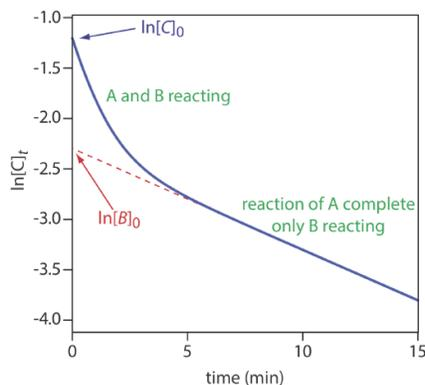
Figure 13.2.15 . Kinetic determination of a slower reacting analyte,  $B$ , in the presence of a faster reacting analyte,  $A$ . The rate constants for the two analytes are:  $k_A = 1 \text{ min}^{-1}$  and  $k_B = 0.1 \text{ min}^{-1}$ .
