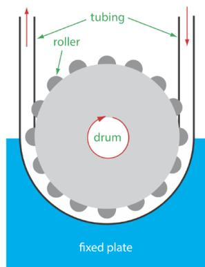
Figure 13.4.7. Schematic diagram of a peristaltic pump.
