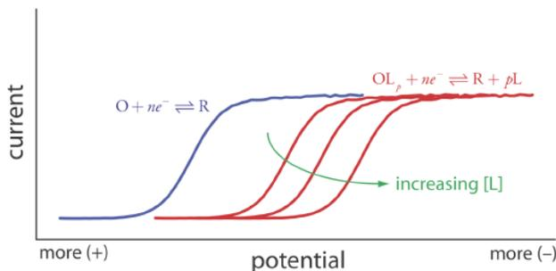
Figure 11.4.21 . Effect of a metal-ligand complexation reaction on a voltammogram. The voltammogram in blue is for the reduction of  $O$  in the absence of ligand. Adding the ligand shifts the potentials to more negative potentials, as shown by the voltammograms in red.
