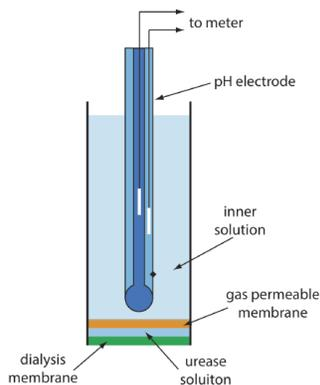
**Figure 11.2.14.** Schematic diagram showing an enzyme-based potentiometric biosensor for urea. A solution of the enzyme urease is trapped between a dialysis membrane and a gas permeable membrane. Urea diffuses across the dialysis membrane and reacts with urease, producing NH<sub>3</sub> that diffuses across the gas permeable membrane. The resulting change in the internal solution's pH is measured with the pH electrode.
