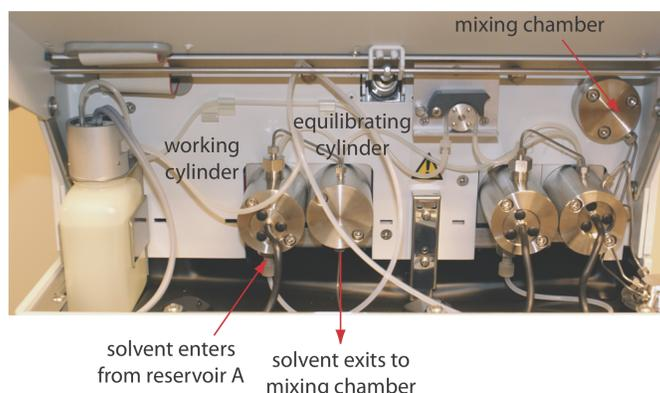
**Figure 12.5.7** . Close-up view of the pumps for the instrument shown in [Figure 12.5.1](#) . The working cylinder and the equilibrating cylinder for the pump on the left take solvent from reservoir A and send it to the mixing chamber. The pump on the right moves solvent from reservoir B to the mixing chamber. The mobile phase's flow rate is determined by the combined speeds of the two pumps. By changing the relative speeds of the two pumps, different binary mobile phases can be prepared.
