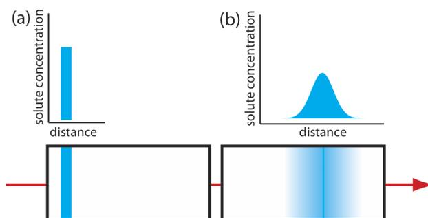
**Figure 12.3.5** . The effect of longitudinal diffusion on a solute's band broadening. Two horizontal cross-sections through the column and the corresponding concentration versus distance profiles are shown, with (a) being earlier in time. The **red** arrow shows the direction in which the mobile phase is moving.
