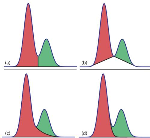
**Figure 12.4.15**. Four methods for determining the areas under two overlapping chromatographic peaks: (a) the drop method; (b) the valley method; (c) the exponential skim method; and (d) the Gaussian skim method. Other methods for determining areas also are available.
