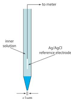
Figure 11.2.19 . Schematic diagram of a liquid-based ion-selective microelectrode.
