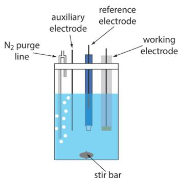
Figure 11.4.4 . Typical electrochemical cell for voltammetry.
