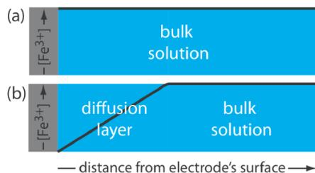
Figure 11.1.2. Concentration of  $\text{Fe}^{3+}$  as a function of distance from the electrode's surface at (a)  $E = +1.00$  V and (b)  $E = +0.500$  V. The electrode is shown in gray and the solution in blue.
