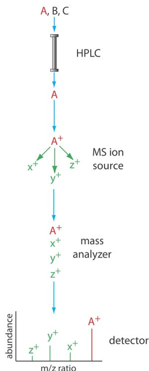
**Figure 12.5.13** . Block diagram of an HPLC–MS. A three component mixture enters the HPLC. When component A elutes from the column, it enters the MS ion source and ionizes to form the **parent ion** and several **fragment ions**. The ions enter the mass analyzer, which separates them by their mass-to-charge ratio, providing the mass spectrum shown at the detector.
