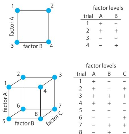
Figure 14.1.12.  $2^k$  factorial designs for (top)  $k = 2$ , and for (bottom)  $k = 3$ . A  $2^2$  factorial design requires four experiments and a  $2^3$  factorial design requires eight experiments.
