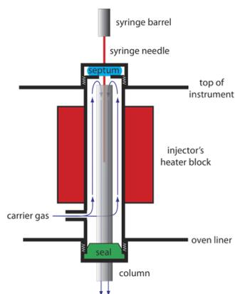
Figure 12.4.7 . Schematic diagram of a heated GC injector port for use with packed columns. The needle pierces a rubber septum and enters into the top of the column, which is located within a heater block.
