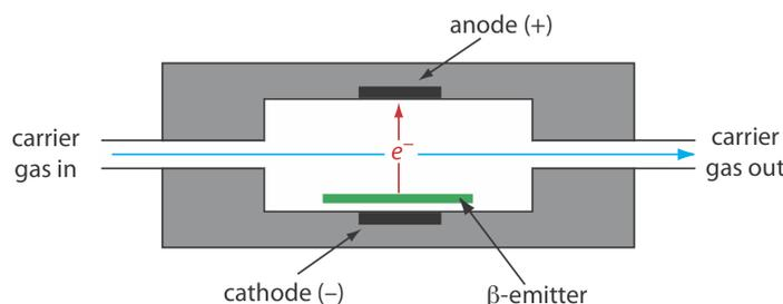
**Figure 12.4.12** . Schematic diagram showing an electron capture detector.
