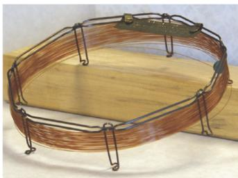
Figure 12.4.3. Typical example of a capillary column for gas chromatography. This column is 30 m long with an internal diameter of 247  $\mu\text{m}$ . The interior surface of the capillary has a 0.25  $\mu\text{m}$  coating of the liquid phase.
