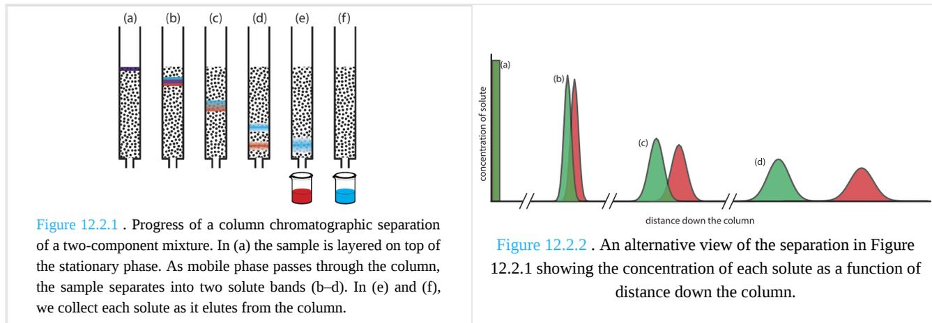
**Figure 12.2.1** . Progress of a column chromatographic separation of a two-component mixture. In (a) the sample is layered on top of the stationary phase. As mobile phase passes through the column, the sample separates into two solute bands (b–d). In (e) and (f), we collect each solute as it elutes from the column.
