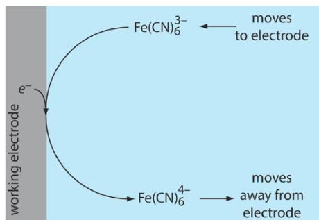
Figure 11.4.6 . Schematic diagram showing the transport of  $\text{Fe}(\text{CN})_6^{4-}$  away from the electrode's surface and the transport of  $\text{Fe}(\text{CN})_6^{3-}$  toward the electrode's surface following the reduction of  $\text{Fe}(\text{CN})_6^{3-}$  to  $\text{Fe}(\text{CN})_6^{4-}$ .
