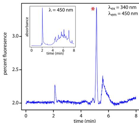
**Figure 12.5.11** . HPLC chromatogram for the determination of riboflavin in urine using fluorescence detection with excitation at a wavelength of 340 nm and detection at 450 nm. The peak corresponding to riboflavin is marked with a red asterisk (\*). The inset shows the same chromatogram when using a less-selective UV/Vis detector at a wavelength of 450 nm. Data provided by Jason Schultz, Jonna Berry, Kaelene Lundstrom, and Dwight Stoll, Department of Chemistry, Gustavus Adolphus College.
