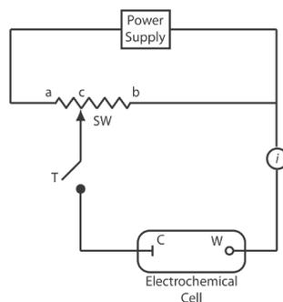
Figure 11.1.3 . Schematic diagram of a manual potentiometer: C is the counter electrode; W is the working electrode; SW is a slide-wire resistor; T is a tap key and  $i$  is an ammeter for measuring current.
