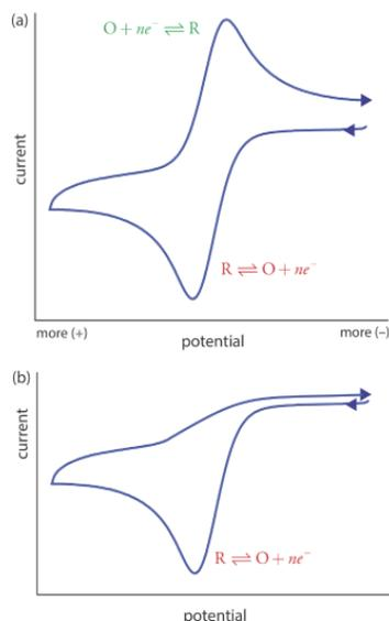
**Figure 11.4.15** . Cyclic voltammograms for  $R$  obtained at (a) a faster scan rate and at (b) a slower scan rate. One of the principal uses of cyclic voltammetry is to study the chemical and electrochemical behavior of compounds. See this chapter's additional resources for further information.
