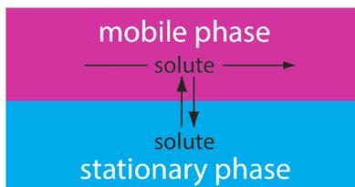
**Figure 12.1.3 .** In chromatography we pass a mobile phase over a stationary phase. When we inject a sample into the mobile phase, the sample’s components both move with the mobile phase and partition into the stationary phase. The solute that spends the most time in the stationary phase takes the longest time to move through the system.
