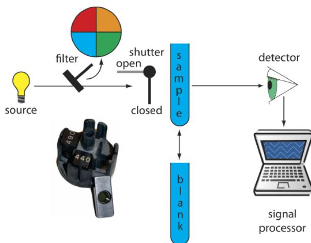
**Figure 10.3.1** . Schematic diagram of a filter photometer. The analyst either inserts a removable filter or the filters are placed in a carousel, an example of which is shown in the photographic inset. The analyst selects a filter by rotating it into place.
