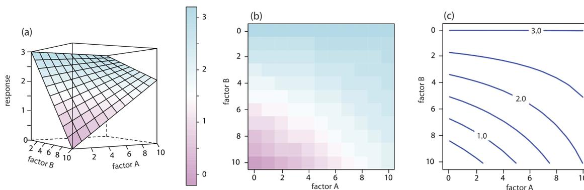
**Figure 14.1.2** . Three examples of a two-factor response surface displayed as (a) a pseudo-three-dimensional wireframe plot, (b) a two-dimensional level plot, and (c) a two-dimensional contour plot. We call the display in (a) a pseudo-three dimensional response surface because we show the presence of three dimensions on the page's flat, two-dimensional surface.
