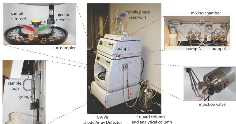
**Figure 12.5.1**. Example of a typical high-performance liquid chromatograph with insets showing the pumps that move the mobile phase through the system and the plumbing used to inject the sample into the mobile phase. This particular instrument includes an autosampler. An instrument in which samples are injected manually does not include the features shown in the two left-most insets, and has a different style of loop injection valve.
