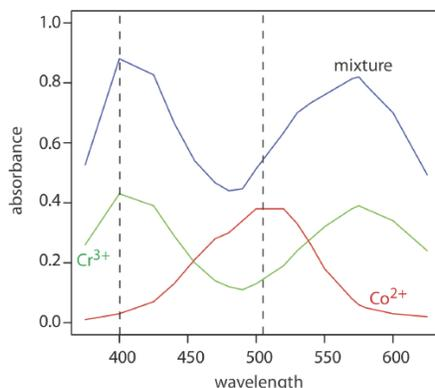
Figure 10.3.11 . Visible absorption spectra for 0.0250 M  $\text{Cr}^{3+}$ , 0.0750 M  $\text{Co}^{2+}$ , and for a mixture of  $\text{Cr}^{3+}$  and  $\text{Co}^{2+}$ . The two wavelengths used to analyze the mixture of  $\text{Cr}^{3+}$  and  $\text{Co}^{2+}$  are shown by the dashed lines. The data for the two standards are from Brewer, S. *Solving Problems in Analytical Chemistry*, John Wiley & Sons: New York, 1980.
