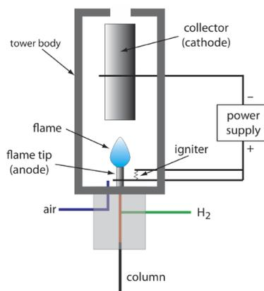
**Figure 12.4.11** . Schematic diagram of a flame ionization detector. The eluent from the column mixes with  $\text{H}_2$  and is burned in the presence of excess air. Combustion produces a flame that contains electrons and the cation  $\text{CHO}^+$ . Applying a potential between the flame's tip and the collector gives a current that is proportional to the concentration of cations in the flame.
