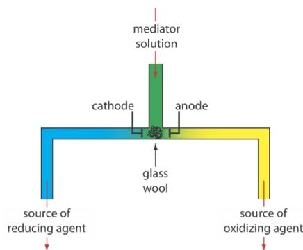
**Figure 11.3.7** . One example of a device for the external generation of oxidizing agents and reducing agents for controlled-current coulometry. A solution containing the mediator flows into a small-volume electrochemical cell. The resulting oxidation products, which form at the anode, flow to the right and serve as an oxidizing agent. Reduction at the cathode generates a reducing agent.
