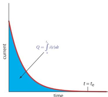
**Figure 11.3.1** . Current versus time for a controlled-potential coulometric analysis. The measured current is shown by the red curve. The integrated area under the curve, shown in blue, is the total charge.
