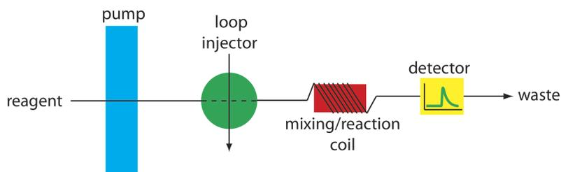
Figure 13.4.8 . Example of a single-channel manifold in which the reagent serves as the carrier stream and as a species that reacts with the sample. The mixing/reaction coil is wrapped around a plastic cylinder.
