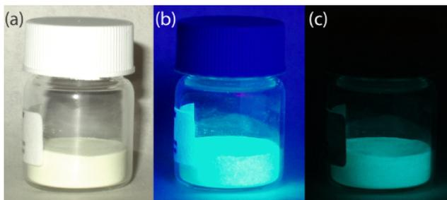
**Figure 10.6.4**. An europium doped strontium silicate-aluminum oxide powder under (a) natural light, (b) a long-wave UV lamp, and (c) in total darkness. The photo taken in total darkness shows the phosphorescent emission. Source: modified from Splarka ([commons.Wikipedia.org](https://commons.wikimedia.org)).
