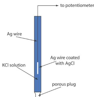
Figure 11.2.6 . Schematic diagram showing a Ag/AgCl electrode. Because the electrode does not contain solid KCl, this is an example of an unsaturated Ag/AgCl electrode.
