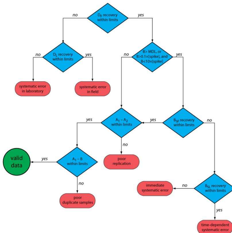
**Figure 15.4.1** . Example of a prescriptive approach to quality assurance for laboratories monitoring waters and wastewaters. Adapted from Environmental Monitoring and Support Laboratory, U. S. Environmental Protection Agency, “Handbook for Analytical Quality Control in Water and Wastewater Laboratories,” March 1979.
