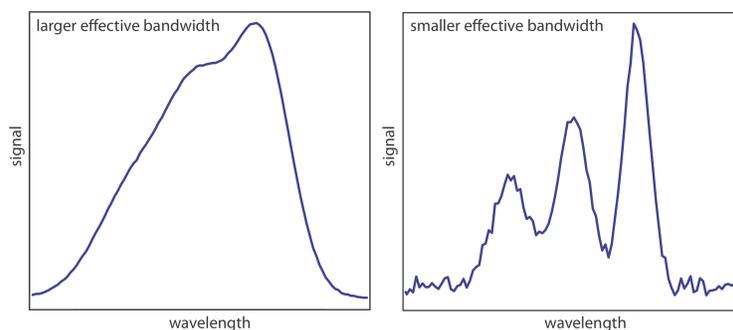
**Figure 10.1.11** . Example showing the effect of the wavelength selector's effective bandwidth on resolution and noise. The spectrum with the smaller effective bandwidth (on the right) has a better resolution, allowing us to see the presence of three peaks, but at the expense of a noisier signal. The spectrum with the larger effective bandwidth (on the left) has less noise, but at the expense of less resolution between the three peaks.
