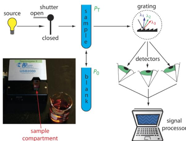
**Figure 10.3.4** . Schematic diagram of a diode array spectrophotometer. The photographic insert shows a typical instrument. Note that the 50-mL beaker provides a sense of scale. Because the spectrometer is small and compact, it is easy to transport into the field.
