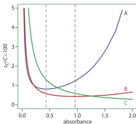
**Figure 10.3.16** . Percent relative uncertainty in concentration as a function of absorbance for the categories of indeterminate errors in Table 1.3.10.3. **A:**  $k_1 = \pm 0.0030$ ; **B:**  $k_2 = \pm 0.0030$ ; and **C:**  $k_3 = \pm 0.0130$ . The dashed lines correspond to the minimum uncertainty for **curve A** (absorbance of 0.4343) and for **curve B** (absorbance of 0.963).
