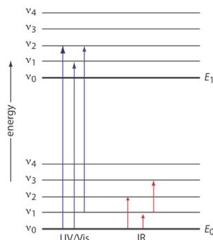
Figure 10.2.1 . Diagram showing two electronic energy levels ( $E_0$  and  $E_1$ ), each with five vibrational energy levels  $\nu_0$ – $\nu_4$ . Absorption of ultraviolet and visible radiation (shown by the blue arrows) leads to a change in the analyte's electronic energy levels and, possibly, a change in vibrational energy as well. A change in vibrational energy without a change in electronic energy levels occurs with the absorption of infrared radiation (shown by the red arrows).
