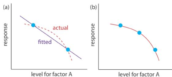
Figure 14.1.15 . A curved one-factor response surface, in red, showing (a) the limitation of using a  $2^1$  factorial design, which can fit only a straight-line to the data, and (b) the application of a  $3^1$  factorial design that takes into account second-order effects.
