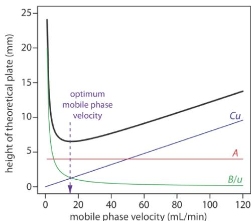
Figure 12.3.7. Plot showing the relationship between the height of a theoretical plate,  $H$ , and the mobile phase's velocity,  $u$ , based on the van Deemter equation.
