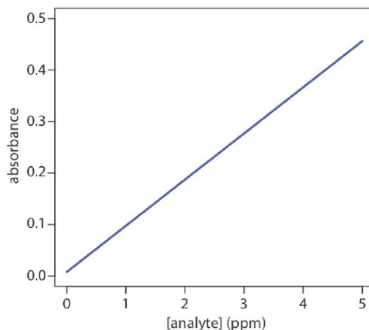
**Figure 14.1.1**. A calibration curve is an example of a one-factor response surface. The responses (absorbance) are plotted on the  $y$ -axis and the factor levels (concentration of analyte) are plotted on the  $x$ -axis.
