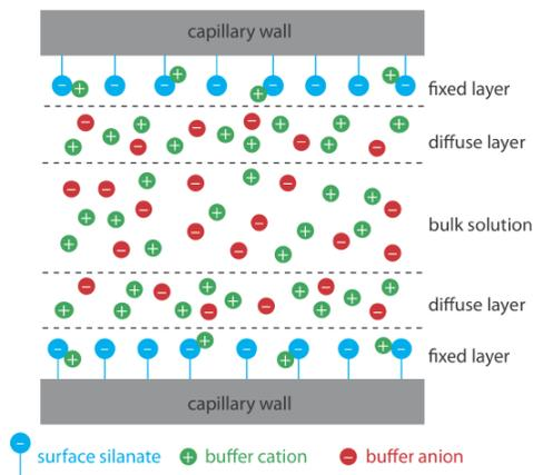
**Figure 12.7.1.** Schematic diagram showing the origin of the double layer within a capillary tube. Although the net charge within the capillary is zero, the distribution of charge is not. The walls of the capillary have an excess of negative charge, which decreases across the fixed layer and the diffuse layer, reaching a value of zero in bulk solution.
