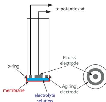
Figure 11.4.16 . Clark amperometric sensor for determining dissolved  $O_2$ . The diagram on the right is a cross-section through the electrode, which shows the Ag ring electrode and the Pt disk electrode.
