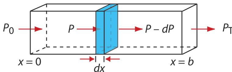
Figure 10.2.8. Factors used to derive the Beer's law.
