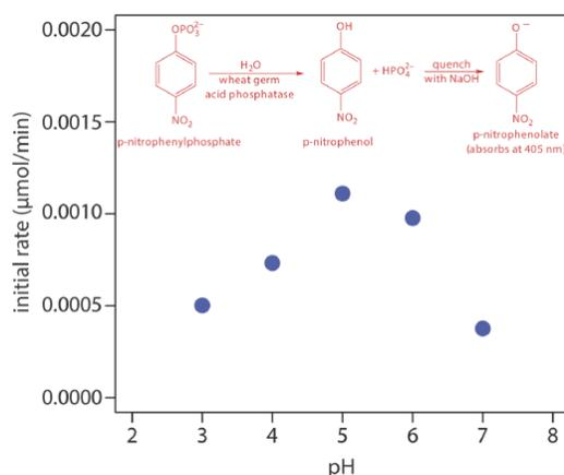
**Figure 13.2.6** . Initial rate for the enzymatic hydrolysis of *p*-nitrophenylphosphate using wheat germ acid phosphatase. Increasing the pH quenches the reaction and converts colorless *p*-nitrophenol to the yellow-colored *p*-nitrophenolate, which absorbs at 405 nm.
