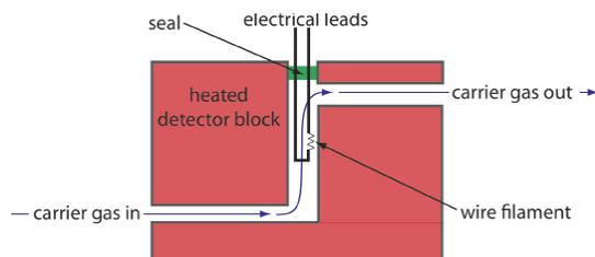
**Figure 12.4.10**. Schematic diagram of a thermal conductivity detector showing one cell of a matched pair. The sample cell takes the carrier gas as it elutes from the column. A source of carrier gas that bypasses the column passes through a reference cell.
