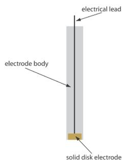
Figure 11.4.3 . Schematic showing a solid electrode. The electrode is fashioned into a disk and sealed in the end of an inert polymer support along with an electrical lead.
