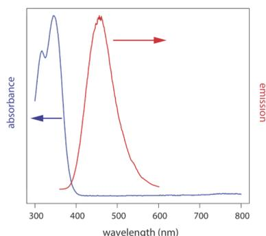
Figure 10.6.5 . Absorbance spectrum and fluorescence emission spectrum for quinine in 0.05 M  $\text{H}_2\text{SO}_4$ . The emission spectrum uses an excitation wavelength of 350 nm with a bandwidth of 20 nm. Both spectra are normalized so that the maximum absorbance is 1.00 and the maximum emission is 1.00. The actual maximum absorbance is 0.444 and the actual maximum emission is 126747. Source: data from Daniel Scott, Department of Chemistry & Biochemistry, DePauw University.
