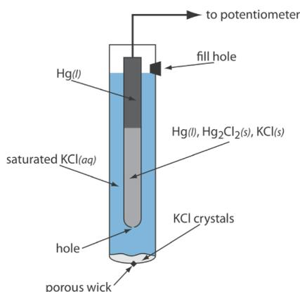
Figure 11.2.5 . Schematic diagram showing the saturated calomel electrode.
