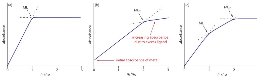
**Figure 10.3.15** . Mole-ratio plots for: (a) a 1:1 metal–ligand complex in which only the complex absorbs; (b) a 1:2 metal–ligand complex in which the metal, the ligand, and the complex absorb; and (c) the stepwise formation of a 1:1 and a 1:2 metal–ligand complex.
