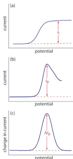
Figure 11.4.9 . The three common shapes for voltammograms. The dashed red line shows the residual current.
