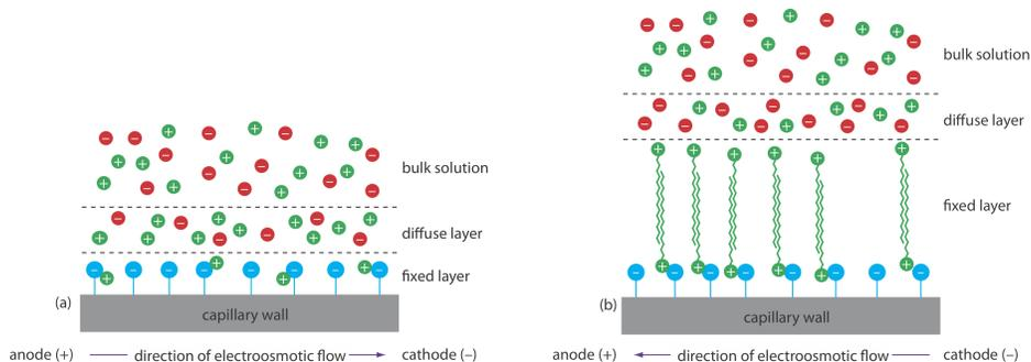
**Figure 12.7.8**. Two modes of capillary zone electrophoresis showing (a) normal migration with electroosmotic flow toward the cathode and (b) reversed migration in which the electroosmotic flow is toward the anode.
