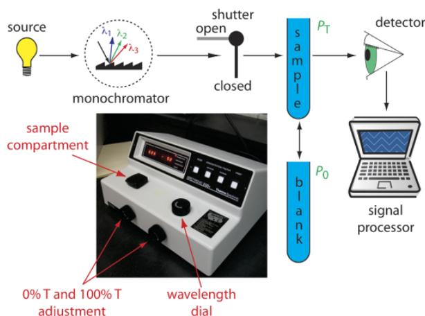
**Figure 10.3.2.** Schematic diagram of a fixed-wavelength, single-beam spectrophotometer. The photographic inset shows a typical instrument. The shutter remains closed until the sample or blank is placed in the sample compartment. The analyst manually selects the wavelength by adjusting the wavelength dial. Inset photo modified from: Adi ([www.commons.Wikipedia.org](http://www.commons.Wikipedia.org)).
