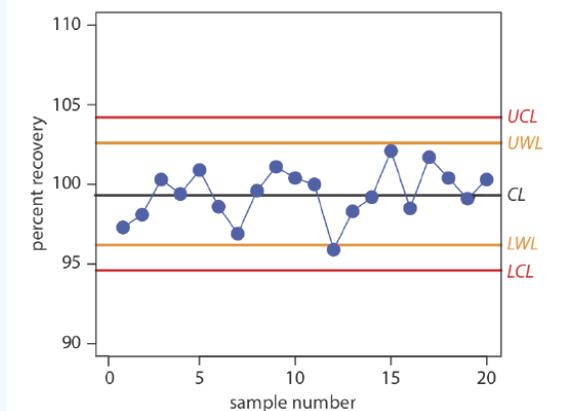
Figure 15.4.2 . Property control chart for Example 15.4.1 . The warning limits are shown in orange and the control limits in red.
