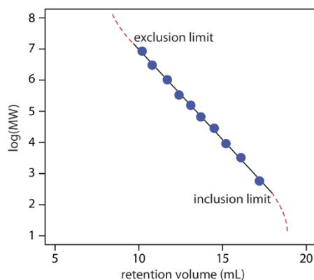
**Figure 12.6.3**. Calibration curve for the determination of molecular weight by size-exclusion chromatography. The data shown here are adapted from Rouessac, F.; Rouessac, A. *Chemical Analysis: Modern Instrumentation Methods and Techniques*, Wiley: Chichester, England, 2004, p 141.
