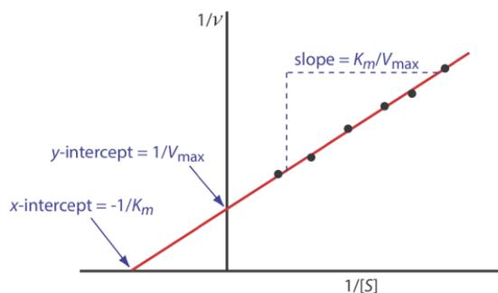
Figure 13.2.10 . Lineweaver–Burk plot of Equation 4.2.25 using Equation ???.
