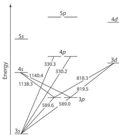
**Figure 10.7.1** . Valence shell energy level diagram for sodium. The wavelengths corresponding to several transitions are shown. Note that this is the same energy level diagram as [Figure 10.2.5](#).
