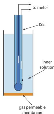
Figure 11.2.13 . Schematic diagram of a gas-sensing membrane electrode.
