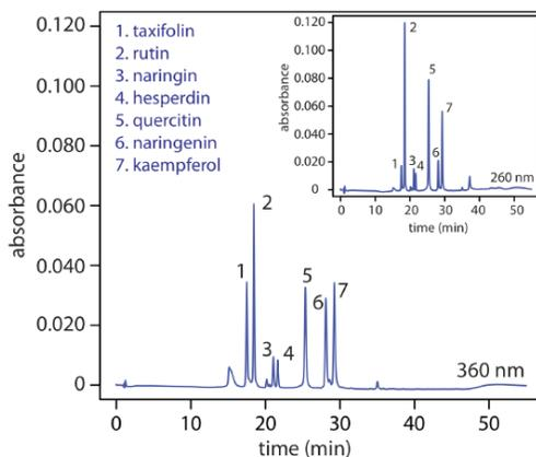
[Figure 12.5.10](#) . HPLC separation of a mixture of flavonoids with UV/Vis detection at 360 nm and, in the inset, at 260 nm. The choice of wavelength affects each analyte's signal. By carefully choosing the wavelength, we can enhance the signal for the analytes of greatest interest. Data provided by Christopher Schardon, Kyle Meinhardt, and Michelle Bushey, Department of Chemistry, Trinity University.
