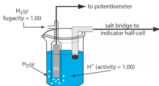
Figure 11.2.4 . Schematic diagram showing the standard hydrogen electrode.
