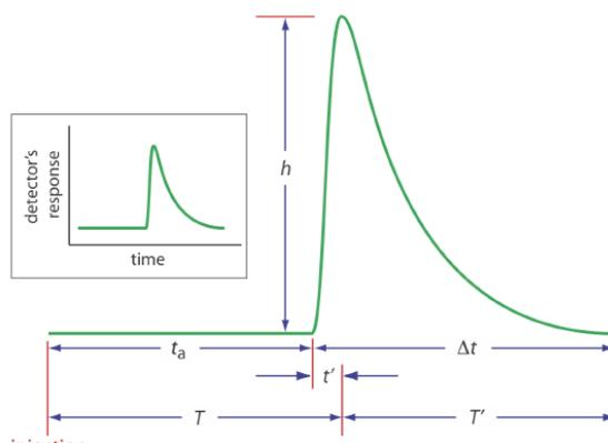
Figure 13.4.4 . Typical fiagram for flow injection analysis showing the detector's response as a function of time. See the text for an explanation of the parameters,  $t_a$ ,  $t'$ ,  $\Delta t$ ,  $T'$ , and  $h$ .
