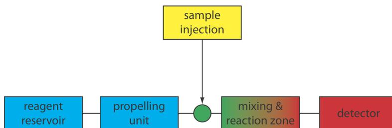
[Figure 13.4.1](#). Schematic diagram of a simple flow injection analyzer showing its basic components. After its injection into the carrier stream the samples mixes and reacts with the carrier stream's reagents before reaching the detector.
