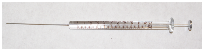
Figure 12.4.8 . Example of a syringe for injecting samples into a gas chromatograph. This syringe has a maximum capacity of 10 \mu\text{L} with graduations every 0.1 \mu\text{L} .
