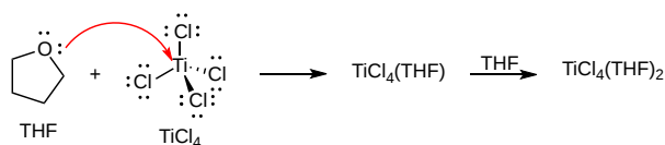
Figure 2.10.2: A Lewis acid-base complex between tetrahydrofuran (THF) and titanium tetrachloride.
