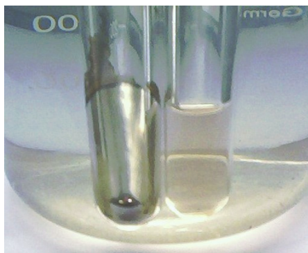
Figure 19.3.2: Tollens test for Aldehyde. The left side is positive (silver mirror) and the right side is negative.
