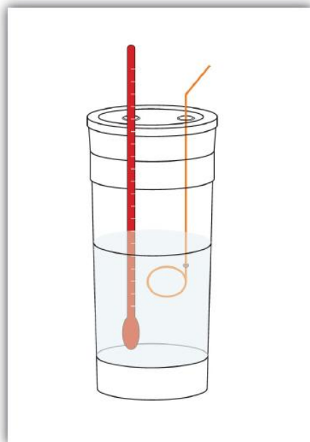
Figure 4.9.2 Calorimeters. A simple calorimeter can be constructed from some nested foam coffee cups, a cover, a thermometer, and a stirrer.
