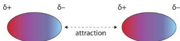
Figure 4.10.1: Dipole-Dipole Interactions. Oppositely charged ends of polar molecules attract each other.
