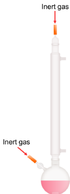
Attaching the condenser to the Schlenk flask.
