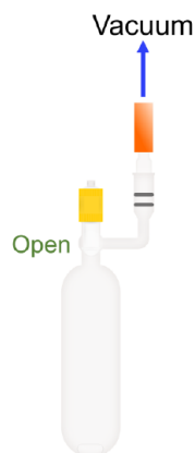
Cycling a Teflon tapped ampoule onto the Schlenk line.
