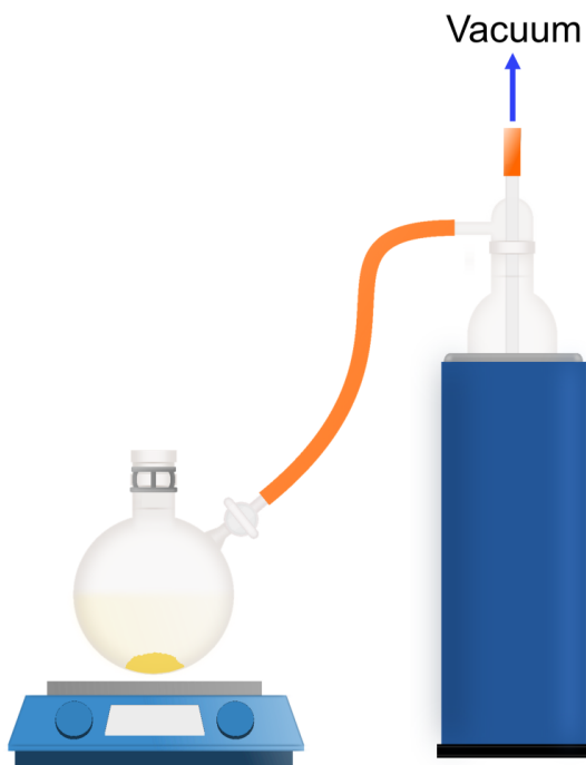
Schlenk flask after removal of solvent.
