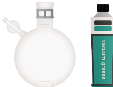
Greased and assembled Schlenk flask.
