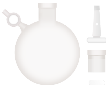
Schlenk flask, stopcock, stopper and stir bar.
