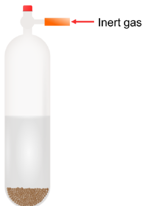
A solvent ampoule ready for cannula transfer.
