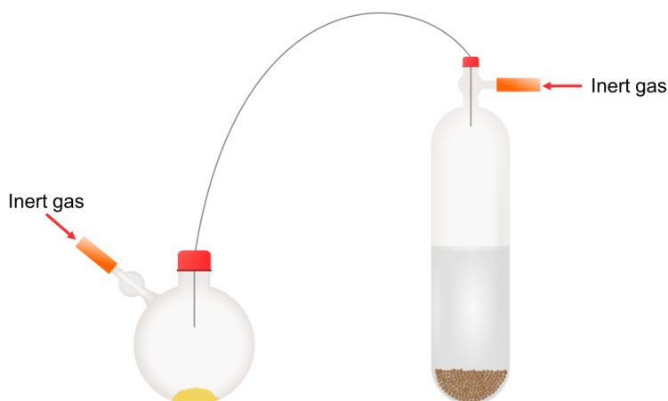
Inserting a cannula into the solvent ampoule and receiving flask.
