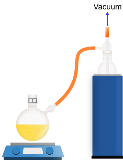
Removing solvent under vacuum.
