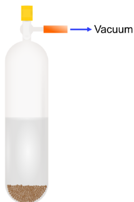
Cycling a solvent ampoule onto the Schlenk line.
