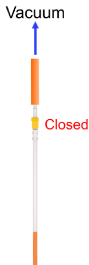
Attaching the NMR tube to the Schlenk line hosing.
