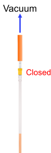
Thawing the contents of the NMR tube under static vacuum.
