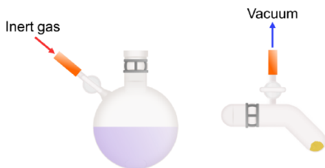
Cycling the solid addition tube onto the Schlenk line.
