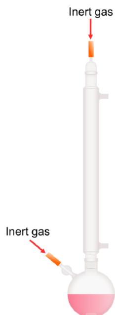
Attaching the condenser to the Schlenk flask.
