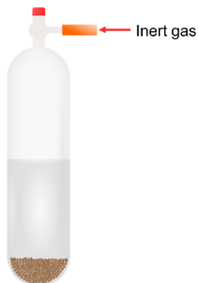
A solvent ampoule ready for cannula transfer.
