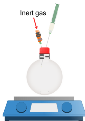
Addition of liquid reagents to the flask.
