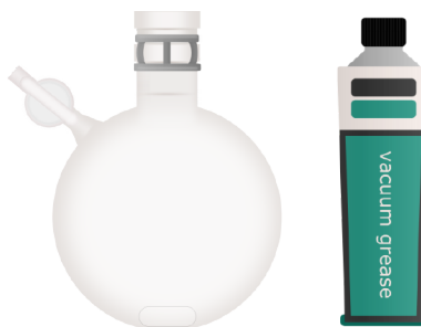
Greased and assembled Schlenk flask.
