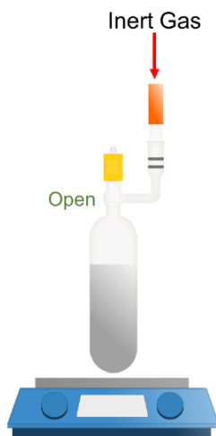
Drying the solvent or liquid reagent over a dessicant.
