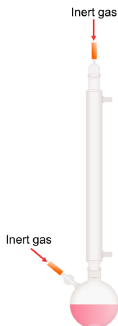
Attaching the condenser to the Schlenk flask.
