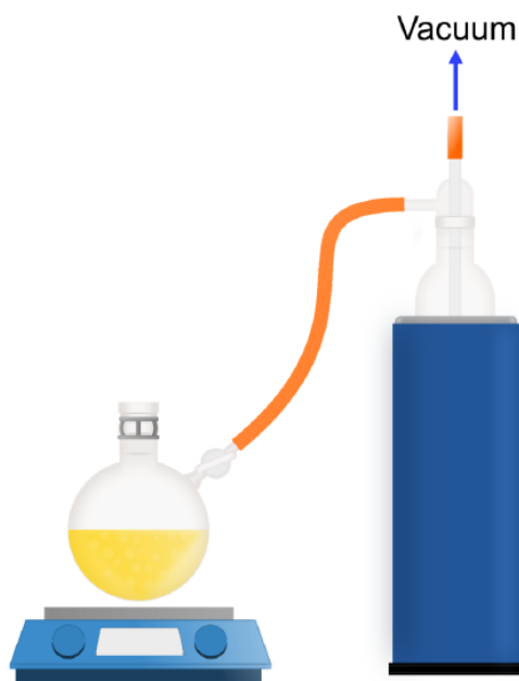
Removing solvent under vacuum.
