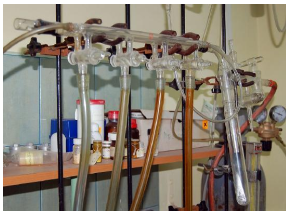
Figure 10.1.1.6: A Schlenk-line ( Polimerek , Double vac line front view , CC BY-SA 3.0 ).
