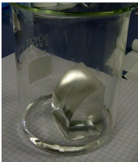
Figure 6.4.4.4: Lithium fluoride (shown here as a large single crystal in a beaker of water) is the only alkali halide that is not freely soluble in water. The lattice energy of LiF is the most negative of the alkali fluorides because \text{Li}^+ and \text{F}^- are both small ions and lattice energy is proportional to 1/r_0 .
