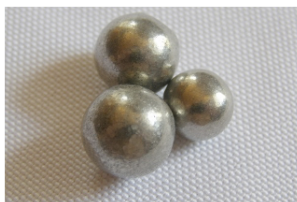
Figure 10.1.1.5: Purified Ni spheres prepared through the Mond process (René Rausch, Nickel kugeln , CC BY-SA 3.0 DE)
