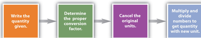
Figure 8.6.2 A Flowchart Illustrating the Steps in Performing a Unit Conversion. When performing many unit conversions, the same logical steps can be taken.
