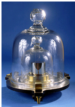
Figure 2.6.2: This replica prototype kilogram is housed at the National Institute of Standards and Technology (NIST) in Maryland. (credit: National Institutes of Standards and Technology).
