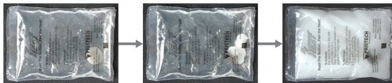
Figure 9.3.10: This hand warmer produces heat when the sodium acetate in a supersaturated solution precipitates. Precipitation of the solute is initiated by a mechanical shockwave generated when the flexible metal disk within the solution is “clicked.” (credit: modification of work by “Velela”/Wikimedia Commons)
