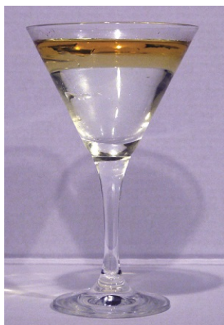
Figure 9.3.7: Water and oil are immiscible. Mixtures of these two substances will form two separate layers with the less dense oil floating on top of the water. (credit: "Yortw"/Flickr)
