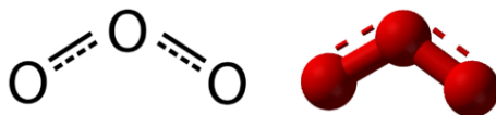
Figure 6.3.2: "Half-bond" model of ozone molecule. This is a better description of the electronic structure of ozone than either of the resonance structures in Figure 6.3.1.
