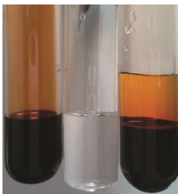
Figure 9.3.8: Bromine (the deep orange liquid on the left) and water (the clear liquid in the middle) are partially miscible. The top layer in the mixture on the right is a saturated solution of bromine in water; the bottom layer is a saturated solution of water in bromine. (credit: Paul Flowers)
