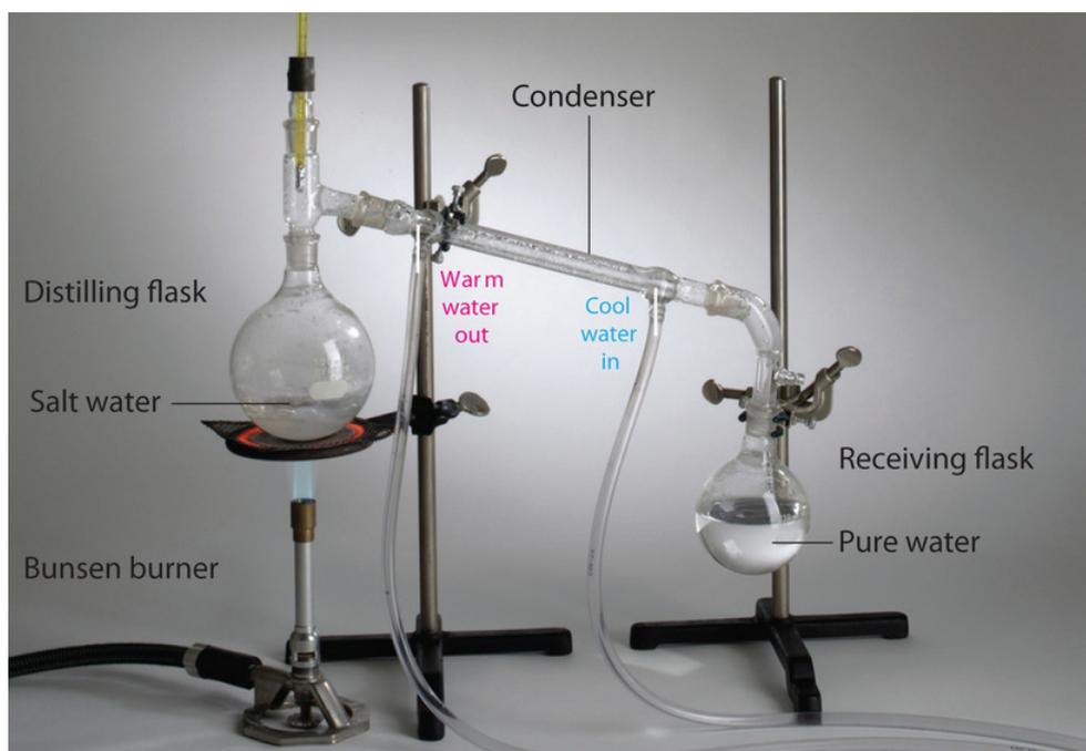
Figure 3.5.3: *The Distillation of a Solution of Table Salt in Water. The solution of salt in water is heated in the distilling flask until it boils. The resulting vapor is enriched in the more volatile component (water), which condenses to a liquid in the cold condenser and is then collected in the receiving flask.*
