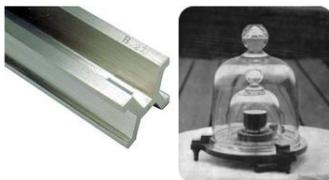
Figure 2.5.1: Meter standard (left) and Kilogram standard (right).
