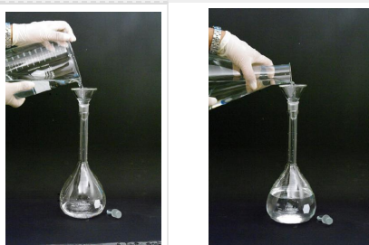
e) The solution is added to volumetric flask by funnel f) Water is added to up the neck of the volumetric flask.
