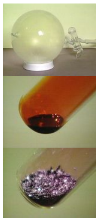
Figure 12.8.1 :The halides show great physical variation . \text{Cl}_2 , a yellow green gas \text{Br}_2 , a red brown liquid \text{I}_2 , a dark crystal
