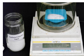
b) 58.441g of NaCl (~1 mole) is measured.
