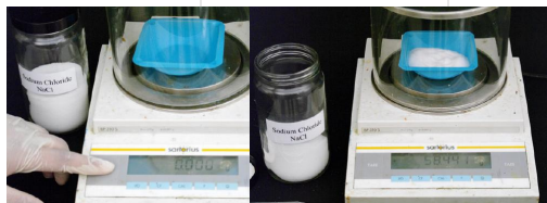
a) a weight boat is zeroed on the balance b) 0.5841 g of NaCl (~1 mole) is measured.
