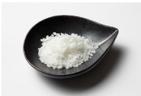
Figure 6.0.3 Table Salt, an example of an ionic compound. Like most ionic compounds, table salt is hard and brittle and dissolves easily in water.
