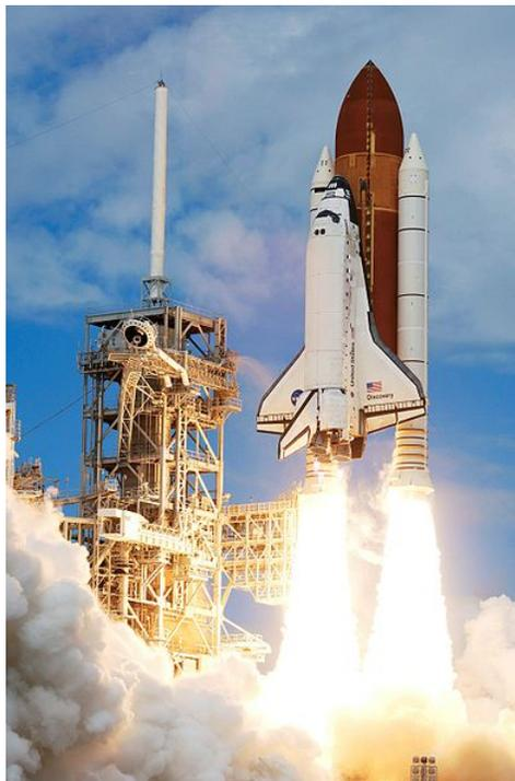
The space shuttle used 2 Solid Propellant Boosters (SRBs, white) and a tank of LOX/LH<sub>2</sub> (large orange tank)
