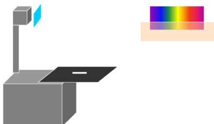
Illustration of a board with a cut out diffraction grating in the center. This board is placed on the lens of a projector. The projecting lens is covered with an opaque film. The resulting spectrum has a continuous spectrum of all the rainbow colors. Red is on the right end and violet is on the left end.
