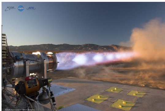
Figure 2. Methane Rocket Engine
