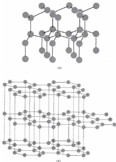
**The crystal structure of (a) diamond and (b) graphite.**
