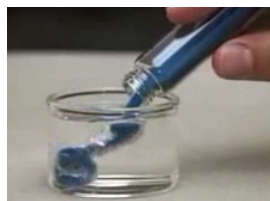
Figure 3: Magic Sand models hydrophobic effect [2]
