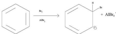
After the electrophilic attack of bromide to the benzene, the hydrogen on the same carbon as bromine substitutes the carbocation in which resulted from the attack. Hence it being an electrophilic aromatic SUBSTITUTION. Since the by-product aluminum tetrabromide is a strong nucleophile, it pulls of a proton from the Hydrogen on the same carbon as bromine.
