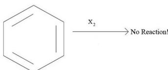
Hence, Halogen needs the help and aid of Lewis Acidic Catalysts to activate it to become a very strong electrophile. Examples of these activated halogens are Ferric Halides (FeX<sub>3</sub>) Aluminum Halides (AlX<sub>3</sub>) where X= Br or Cl. In the following examples, the halogen we will look at is Bromine.
