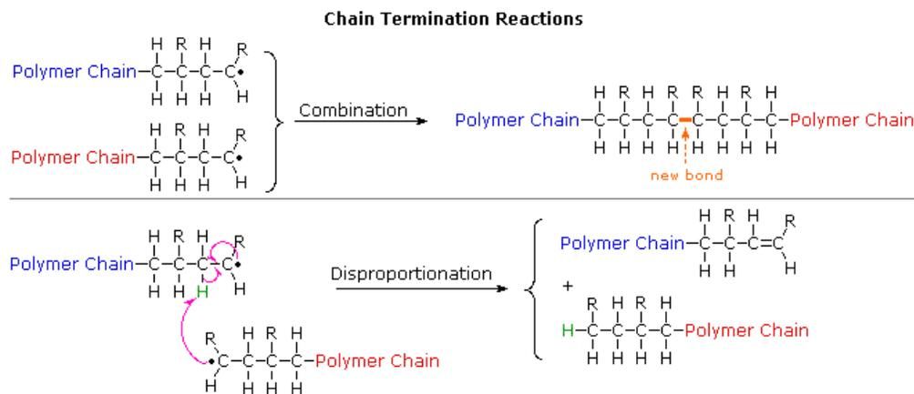
The relative importance of these terminations varies with the nature of the monomer undergoing polymerization. For acrylonitrile and styrene combination is the major process. However, methyl methacrylate and vinyl acetate are terminated chiefly by disproportionation.
