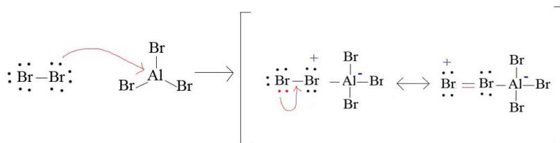
As the bromine has now become more electrophilic after activation of a catalyst, an electrophilic attack by the benzene occurs at the terminal bromine of Br-Br-AlBr<sub>3</sub>. This allows the other bromine atom to leave with the AlBr<sub>3</sub> as a good leaving group, AlBr<sub>4</sub><sup>-</sup>.
