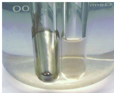
Figure 5.4.1: Tollens test for Aldehyde: Left Side Positive (silver mirror), Right Side Negative
