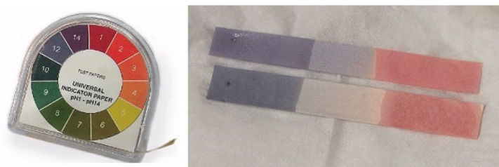
Figure 3.3.9: pH Paper. pH paper contains a set of indicators that change color at different pH values. The approximate pH of a solution can be determined by simply dipping a paper strip into the solution and comparing the color to the standards provided. (CC BY-SA-NC; Anonymous by request)
