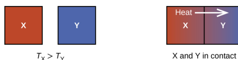
Figure 1.1.4: When two objects at different temperatures come in contact, heat spontaneously flows from the hotter to the colder object. Two separated blocks. One is labeled X and the other labeled Y. The diagram next to it shows the two blocks in contact with one another.
