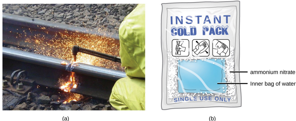
Figure 2.2.1.6: (a) An oxyacetylene torch produces heat by the combustion of acetylene in oxygen. The energy released by this exothermic reaction heats and then melts the metal being cut. The sparks are tiny bits of the molten metal flying away. (b) A cold pack uses an endothermic process to create the sensation of cold. (credit a: modification of work by “Skatebiker”/Wikimedia commons)
