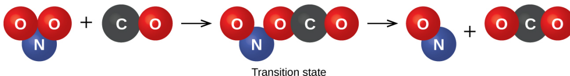
Figure 2.3.6.1: The probable mechanism for the reaction between NO_2 and CO to yield NO and CO_2 .
