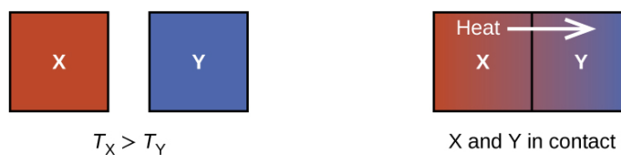
Figure 2.2.3.4: When two objects at different temperatures come in contact, heat spontaneously flows from the hotter to the colder object.
