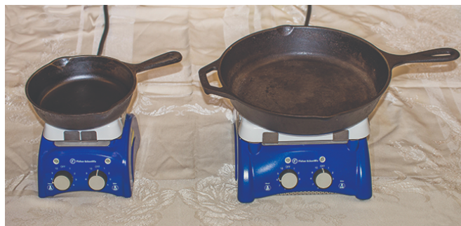
Figure 2.2.1.7: Because of its larger mass, a large frying pan has a larger heat capacity than a small frying pan. Because they are made of the same material, both frying pans have the same specific heat. (credit: Mark Blaser)
