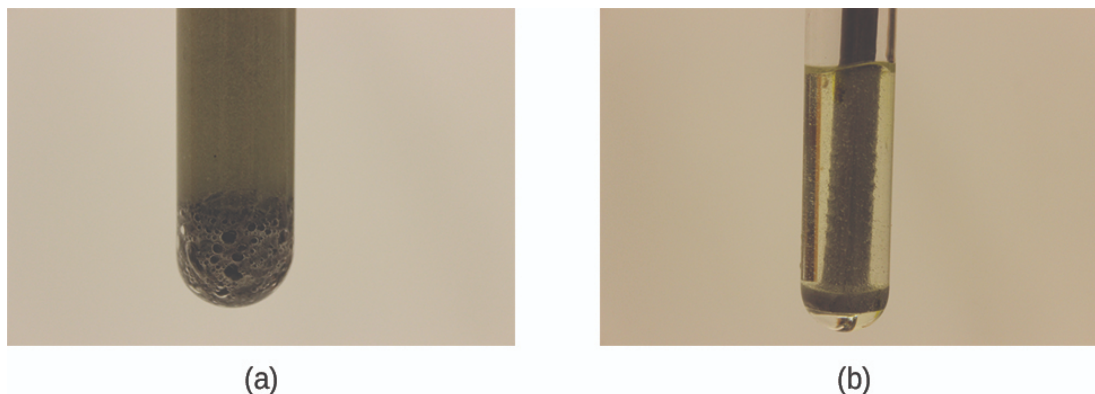
Figure 2.3.2.1: (a) Iron powder reacts rapidly with dilute hydrochloric acid and produces bubbles of hydrogen gas: 2\text{Fe(s)} + 6\text{HCl(aq)} \rightarrow 2\text{FeCl}_3\text{(aq)} + 3\text{H}_2\text{(g)} . (b) An iron nail reacts more slowly because the surface area exposed to the acid is much less.
