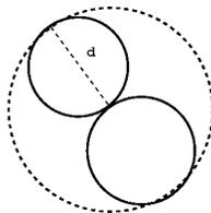
If we consider two hard spheres at closest contact and draw the smallest imaginary sphere that contains both particles, then we find this latter sphere has a radius  $u_0(r)$ :
