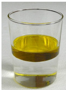
Figure 1.9.1.2: Water (clear liquid) and oil (yellow) do not form liquid solutions. (CC BY-SA 1.0 Generic; Victor Blacus)
