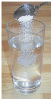
Figure 1.9.1.1: Making a saline water solution by dissolving table salt (NaCl) in water. The salt is the solute and the water the solvent. (CC-BY-SA 3.0; Chris 73 ).
