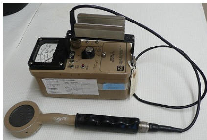
Figure 1.5.4.1: Detecting Radioactivity. A Geiger counter is a common instrument used to detect radioactivity.
