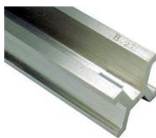
Figure 1.1.6.1: Meter Standard. (Credit: Courtesy of U.S. Department of Commerce; Courtesy of National Institute of Standards and Technology; Source: http://commons.wikimedia.org/wiki/File:US_National_Length_Meter.JPG (opens in new window); http://commons.wikimedia.org/wiki/File:Standard_kilogram,_2.jpg (opens in new window); License: Public Domain)
