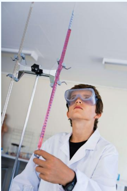
Figure 1.9.7.1.1 Titration © Thinkstock. When a student performs a titration, a measured amount of one solution is added to another reactant.
