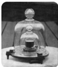
Figure 1.1.6.2: Kilogram standard (Credit: Courtesy of National Institute of Standards and Technology; Source: http://commons.wikimedia.org/wiki/File:Standard_kilogram,_2.jpg (opens in new window); License: Public Domain)
