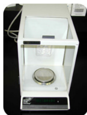
Figure 1.1.6.2.2: An analytical balance makes very sensitive mass measurements in a laboratory, usually in grams. (Credit: Courtesy of US Drug Enforcement Administration; Source: http://commons.wikimedia.org/wiki/File:Analytical_balance_mettler_ae-260.jpg (opens in new window); License: Public Domain)
