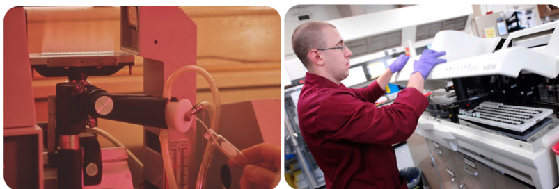
Figure 1.1.1.2: (left) Measurement of trace metals using atomic spectroscopy. (right) Measurement of hormone concentrations.
