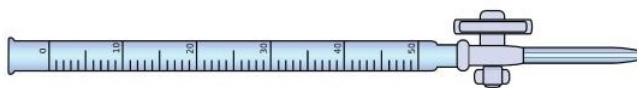
Figure 1.11.8.1: Equipment for Titrations. A burette is a type of liquid dispensing system that can accurately indicate the volume of liquid dispensed.
