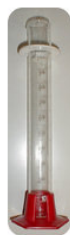
Figure 1.1.6.1.4: A graduated cylinder is often used to measure volume in the laboratory, and comes in a variety of sizes. (Credit: User:Darrien/Wikipedia; Source: http://commons.wikimedia.org/wiki/File:Graduated_cylinder.jpg (opens in new window); License: Public Domain)
