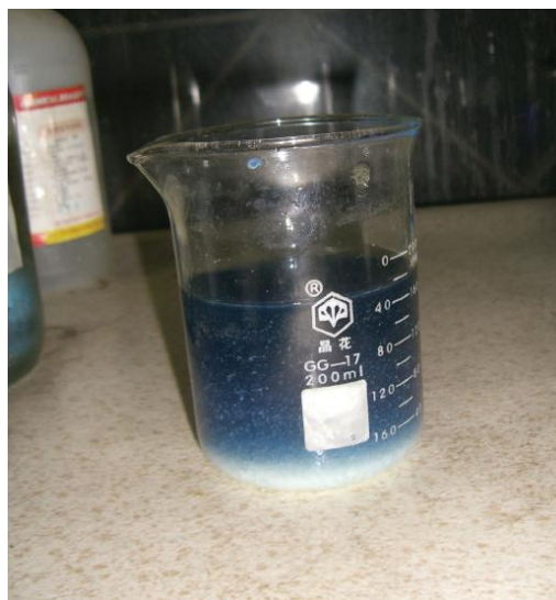
Figure 1.7.4.2: Double-Replacement Reactions. Some double-replacement reactions are obvious because you can see a solid precipitate coming out of solution. Source: Photo courtesy of Choij, http://commons.wikimedia.org/wiki/File:Copper_solution.jpg (opens in new window).
