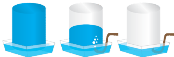
Figure 1.8.8.2: A gas produced in a chemical reaction can be collected by water displacement.
