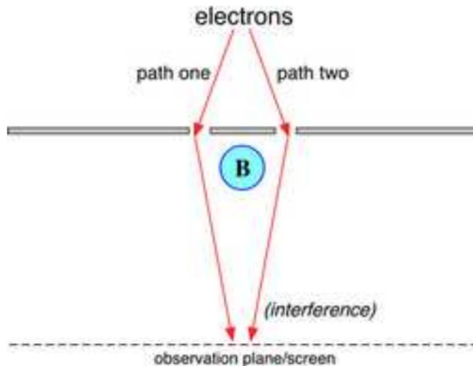
Schematic of double-slit experiment in which Aharonov–Bohm effect can be observed: electrons pass through two slits, interfering at an observation screen, with the interference pattern shifted when a magnetic field  $\mathbf{B}$  is turned on in the cylindrical solenoid. (All of the above adapted from Wikipedia)
