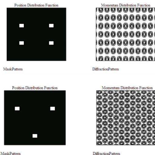
Clearly both diffraction patterns exhibit translational periodicity, their repeating units being a 90 degree rotation of the spatial structure. Next we look at four-fold rotational symmetry and see that the unit cell is obvious.
