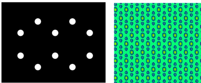
This calculation illustrates the uncertainty principle. There is no attenuation in the diffraction pattern (momentum distribution) because there is no uncertainty in the carbon atom positions.
