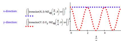
For the MZ polarization interferometer diagonally polarized light enters in the x-direction,  $|x\rangle$ . Tensor vector multiplication is awkward in Mathcad as shown below.
