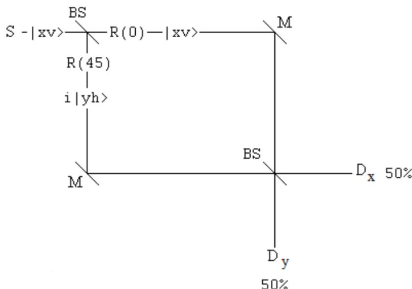
Photon behavior in the absence of the polarization rotator in the lower arm of the interferometer.
