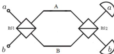
Because the photons are indistinguishable they don't possess separate identities, and we are forced by quantum mechanical principles to represent their collective state at the beam splitter (BS) by the following entangled wave function. The plus sign in this superposition indicates that photons are bosons; their wave functions are symmetric with respect to the interchange of the photon labels.
