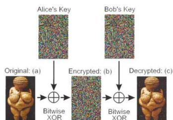
By extending the previous example to two dimensions, it is easy to produce a rudimentary simulation of the experiment. Bitwise XOR is nothing more than addition modulo 2. (XOR = CNOT)
