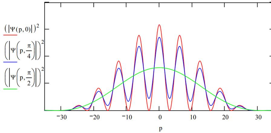
We see that when the polarizers are oriented at the same angle, the diffraction pattern is the usual one for the Young double-slit experiment. When the polarizers are crossed the fringes, as Fresnel and Arago assert, disappear. Finally, when the relative angle of the two polarizers is 45 degrees, we see a reduced interference pattern.
