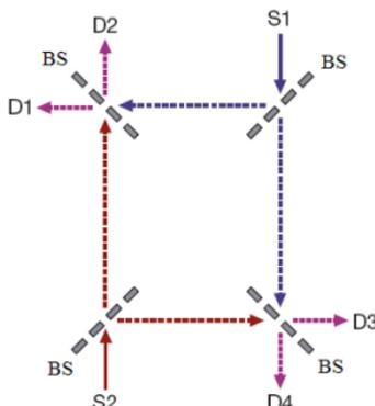
S1 and S2 are the electron sources, BS labels the four 50-50 beam splitters and D1, D2, etc. are the electron detectors.
