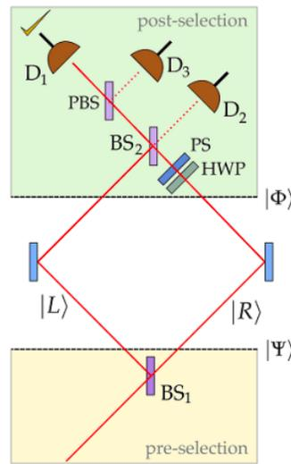
In the absence of the half-wave plate (HWP) and the phase shifter (PS) a horizontally polarized photon entering the interferometer from the lower left (propagating to the upper right) arrives at  $D_2$  with a 90 degree ( $\pi/2$ ,  $i$ ) phase shift. (By convention reflection at a beam splitter introduces a 90 degree phase shift.)
