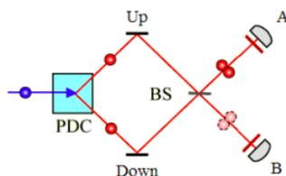
A parametric down converter, PDC, transforms an incident photon into two lower energy photons. One photon takes the upper path and the other the lower path or vice versa. The principles of quantum mechanics require that the wave function for this event be written as the following entangled superposition.
