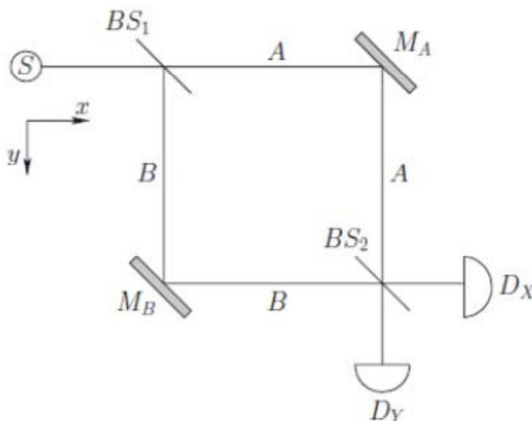
A key convention in the analysis of MZ interferometers is that reflection at a beam splitter (BS) is accompanied by a 90 degree phase shift ( $\frac{\pi}{2}$ ,  $i$ ). The behavior of a photon traveling in the x- or y-direction at the beam splitters and mirrors is as follows.
