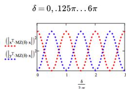
Demonstrate that a superposition is formed after the first beam splitter.
