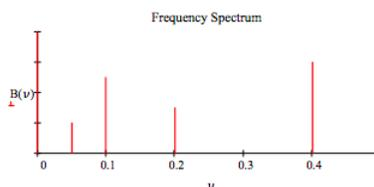
This calculation reveals how a Michelson interferometer is used to measure the wavelengths or frequencies present in the source beam. In a FT-IR instrument the source ideally contains all the IR frequencies. The sample is placed between the beam splitter and the detector and an absorption spectrum is measured.
