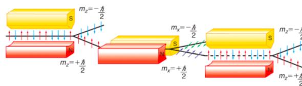
Silver atoms are deflected by an inhomogeneous magnetic field because of the two-valued magnetic moment associated with their unpaired 5s electron ( $[\text{Kr}]5s^14d^{10}$ ). The beam of silver atoms entering the Stern-Gerlach magnet oriented in the z-direction (SGZ) on the left is unpolarized. This means it is a mixture of randomly polarized Ag atoms. A mixture cannot be represented by a wave function, it requires a density matrix, as will be shown later.
