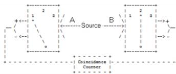
The switches on the detectors are set randomly so that all nine possible settings of the two detectors occur with equal frequency.
