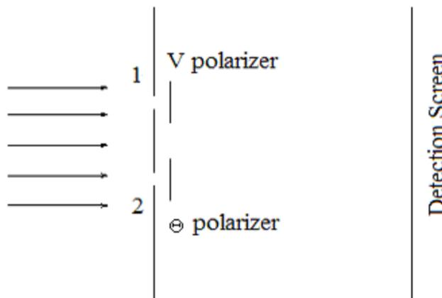
Assuming infinitesimally thin slits, the photon wave function is a superposition of being at slit 1 with vertical polarization and slit 2 with polarization at an angle  $\theta$  relative to the vertical.
