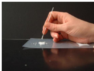
Figure 5.2.5. Loading a capillary tube with aspirin
