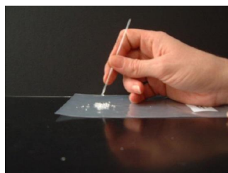
Figure 5.2.5. Loading a capillary tube with aspirin
