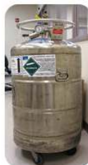
Figure 13.5.3: Helium gas liquefies at 4 K, or four degrees above absolute zero. Liquid helium is used as a coolant for large superconducting magnets, and must be stored in insulated metal canisters. (CC BY 2.0; Michael Pereckas (Flickr: Beige Alert) via Flickr)
