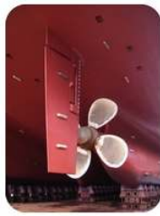
Figure 22.5.2: Small blocks of zinc are attached to the steel hull of this ship.
