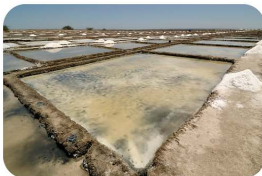
Figure 2.10.3: Once the sea water in these evaporation ponds has evaporated, the salt can be harvested. (CC BY 3.0; Sandip Dey (Wikimedia: Dey.sandip) via Commons Wikimedia, Salt pans in Marakkanam, India [commons.wikimedia.org])
