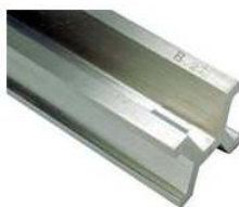
Figure 3.1.1: Meter Standard. (Public Domain; US Department of Commerce; National Institute of Standards and Technology via Wikipedia; http://commons.wikimedia.org/wiki/File:Standard_kilogram,_2.jpg )
