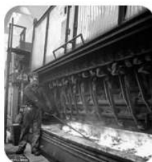
Figure 2.14.1: Electrolytic production of aluminum. (Public Domain; Ronny Jacques via Wikipedia )
