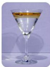
Figure 15.6.1: Water and oil form separate layers when they are mixed because the nonpolar oil will not dissolve into the polar water. The oil forms the top layer because it is less dense than the water.
