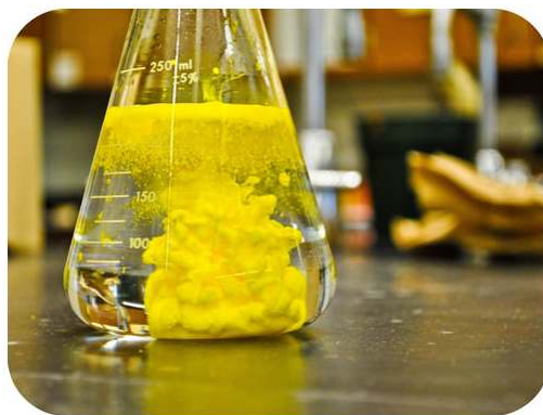
Figure 2.18.4: A yellow precipitate of solid lead (II) iodide forms immediately when solutions of lead (II) nitrate and potassium iodide are mixed. (CC by 2.0; Paige Powers (Flickr: paigggeyy) via Flickr )
