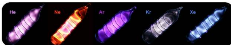
Figure 5.5.2: Gas discharge tubes are enclosed glass tubes filled with a gas at low pressure, through which an electric current is passed. Electrons in the gaseous atoms first become excited, and then fall back to lower energy levels, emitting light of a distinctive color in the process. Shown are gas discharge tubes of helium, neon, argon, krypton, and xenon. (CC by 3.0; User:Jurii/Wikimedia Commons, Heinrich Pniok (Wikimedia: Alchemist-hp) via Commons Wikimedia, Glowing noble gases [commons.wikimedia.org])
