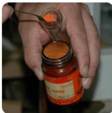
Figure 11.5.2: Mercury (II) oxide is a red solid. When it is heated, it decomposes into mercury metal and oxygen gas. (Public Domain; Ben Mills (User:Benjah-bmm27/Wikimedia Commons) via Wikipedia )
