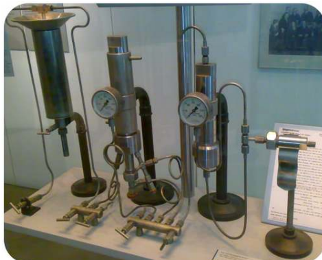
Figure 12.2.4: An apparatus for running the Haber process. (Public Domain; User: JGvBerkel/Wikimedia Commons via Commons Wikimedia, Haber Ammonia [commons.wikimedia.org])
