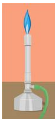
Figure 11.1.3: A Bunsen burner is commonly used to heat substances in a chemistry lab. Methane is reacted with oxygen to form carbon dioxide and water. (CK-12 Curriculum Materials license; CK-12 Foundation via CK-12 Foundation)
