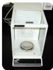
Figure 3.5.2: An analytical balance makes very sensitive mass measurements in a laboratory, usually in grams. (Public Domain; U.S. Drug Enforcement Administration via Wikipedia )
