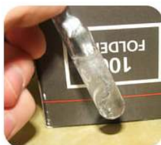
Figure 2.18.3: Zinc reacting with hydrochloric acid produces bubbles of hydrogen gas. (Public Domain; User:Chemicalinterest/Wikimedia Commons via Wikipedia )
