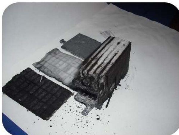
Figure 23.7.2: A lead storage battery, such as those used in cars, consists of six identical electrochemical cells and is rechargeable.
