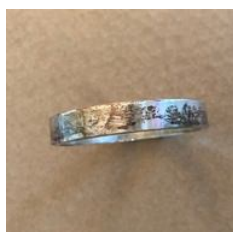
Figure 11.1.2: You can see dark spots of tarnished (silver sulfide) forming on this ring as it reacts with sulfur compounds in the air. (CK-12 Curriculum Materials license; CK-12 Foundation via CK-12 Foundation)
