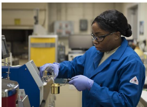
Figure 1.5.1: U.S. Air Force Technical Sergeant Shanice Spearman at Aerospace Fuels Laboratory NCO prepares fuel samples for flashpoint testing. (Public Domain; Airman 1st Class Greg Erwin via https://www.kadena.af.mil/News/Photo...oto/2001869405 )
