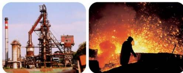
Figure 22.9.1: A blast furnace is where iron ore is processed and turned into iron metal. First, air is blown through a mixture of iron ore and coke (carbon). The carbon monoxide produced reduces the \text{Fe}^{3+} ions in the iron ore to metallic iron.
