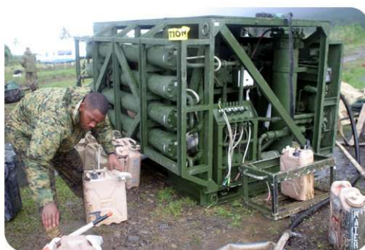
Figure 1.8.2: Desalination equipment. (Lance Cpl. Willard J. Lathrop, U.S. Marine Corps; Source: http://commons.wikimedia.org/wiki/File:US_Navy_06022014_Equipment_Specialist_Cpl_Xzavia_Granger_assigned_to_the_31st_Marine_Expeditionary_Unit_%2528MEU%2529_Service_Support_Group_31,_prepares_a_chlorine_gas_cylinder ; License: Public Domain)
