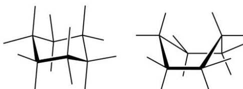
Figure 25.6.2: Chair (left) and boat (right) conformations for cyclohexane.
