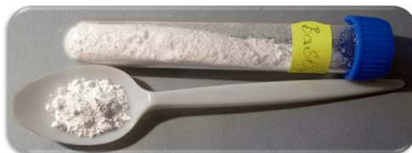
Figure 19.14.1: Barium sulfate is used as a component of white pigment for paints and as an agent in certain x-ray imaging processes.
