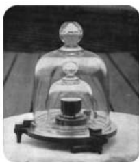
Figure 3.1.2: Kilogram standard (Public Domain; National Institute of Standards and Technology via Wikipedia)
