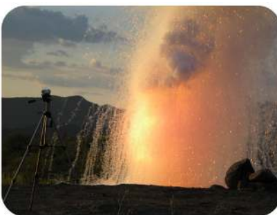
Figure 11.7.3: Sodium metal reacts vigorously with water, giving off hydrogen gas. A large piece of sodium will often generate so much heat that the hydrogen will ignite. (Public Domain; User:Ajhalls/Wikimedia Commons via Wikipedia )
