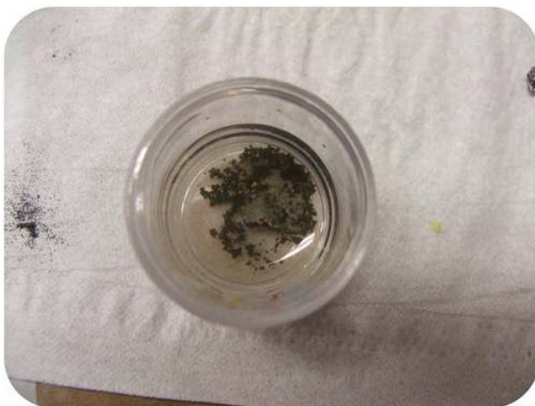
Figure 23.1.2: Reaction of zinc metal in copper sulfate solution.
