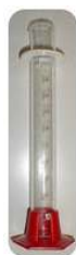
Figure 3.4.4: A graduated cylinder is often used to measure volume in the laboratory, and comes in a variety of sizes. (Public Domain; User:Darrien/Wikipedia via Wikipedia )
