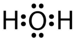
Figure 9.15.4: Lone pair electrons on water. (CC BY-NC 3.0; Joy Sheng via CK-12 Foundation)
