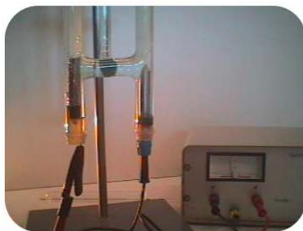
Figure 23.9.1: Apparatus for the production of hydrogen and oxygen gases by the electrolysis of water.
