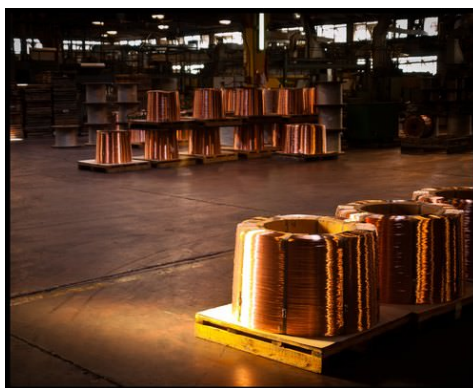
Figure 9.1.3: Metallic bonds explain many of the properties of metals. This coil of wire is made of the metal copper. Like other metals, copper is shiny, can be formed into wires, and conducts electricity. (CC BY 2.0; Flavio~ - "Industrial Photography: Copper Wires-003" via Flickr)
