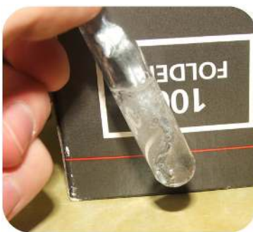
Figure 11.7.2: Zinc metal reacts with hydrochloric acid to give off hydrogen gas in a single-displacement reaction. (Public Domain; User: Chemicalinterest/Wikimedia Commons via Wikipedia )
