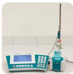
Figure 21.14.1: A pH meter is a laboratory device that provides quick, accurate measurements of the pH of solutions. (CC BY-NC; CK-12)
