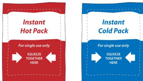
Figure 17.13.1: Chemical hot packs and cold packs work because of the heats of solution of the chemicals inside them. When the bag is squeezed, an inner pouch bursts, allowing the chemical to dissolve in water. Heat is released in the hot pack and absorbed in the cold pack. (CC BY-NC; CK-12)
