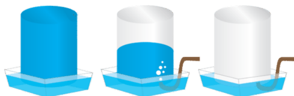
Figure 14.13.1: A gas produced in a chemical reaction can be collected by water displacement. (CC BY-NC; CK-12)
