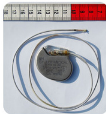
Figure 6.14.5: Pacemaker. (CC BY 3.0; Steven Fruitsmaak via Commons Wikimedia, St. Jude Medical Pacemaker with Ruler [commons.wikimedia.org])
