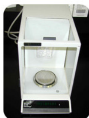
Figure 3.5.2: An analytical balance makes very sensitive mass measurements in a laboratory, usually in grams. (Public Domain; U.S. Drug Enforcement Administration via Wikipedia )
