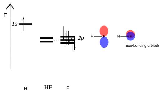
5. The H 1s and F 2p<sub>z</sub> make a bonding and anti-bonding combination, so we draw these new MO energy levels. We don't know exactly how big the splitting is, but that's ok, don't worry about it.
