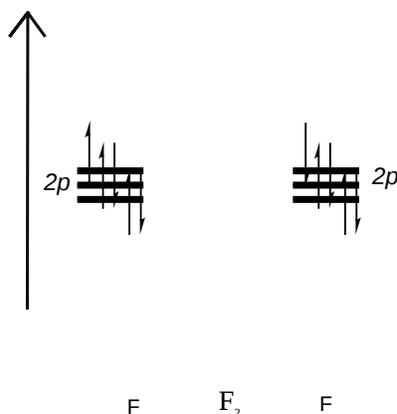
4. We remember which orbitals interact. Before, we saw that we make  $\sigma$  bond and anti-bonding combinations using the 2p orbitals that point toward each other. Let's draw those in.
