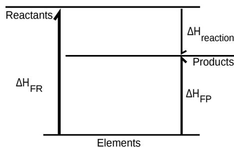
A diagram showing the application of Hess' law to reaction enthalpy calculated from enthalpies of formation.
