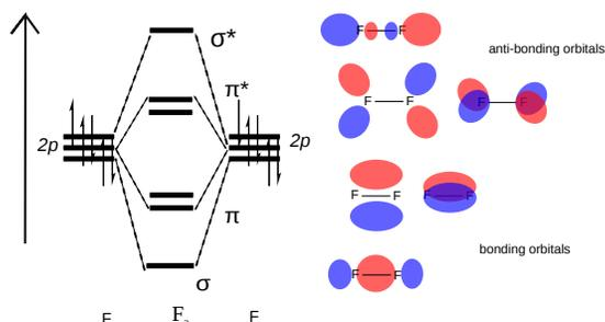
6. We put the same number of valence electrons we had in the AOs on the outside into the MOs at the center. In this case, we have 10 electrons. They will go into the  $\sigma$  bonding MO and all 4  $\pi$  MOs. Only the  $\sigma^*$  MO is left empty. We're done!
