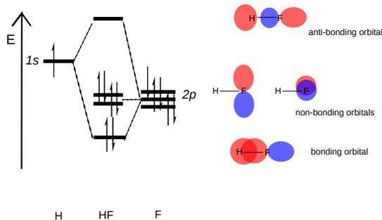
MO diagram for HF. Notice that the bond order is 1, as we expect from the Lewis structure (2 electron in bonding MO, 4 electrons in non-bonding MOs).
