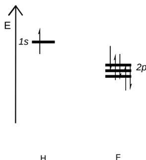
4. We remember which orbitals interact. Before, we saw that bonding and anti-bonding combinations only form between H 1s and the F 2p orbital that points straight toward it. The other 2p orbitals are non-bonding, so we can draw them in the middle at the same starting energy.
