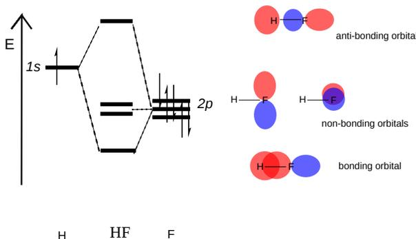
6. We put the same number of valence electrons we had in the AOs on the outside into the MOs at the center, starting at the bottom. In this case, we have 6 electrons. They will go into the bonding MO and the 2 non-bonding MOs. The anti-bonding MO is empty because it is too high in energy. We're done!
