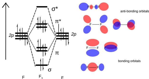
MO diagram for  $F_2$ . Notice that the bond order is 1, as we expect from the Lewis structure (6 electrons in bonding MOs, 4 electrons in anti-bonding MOs).
