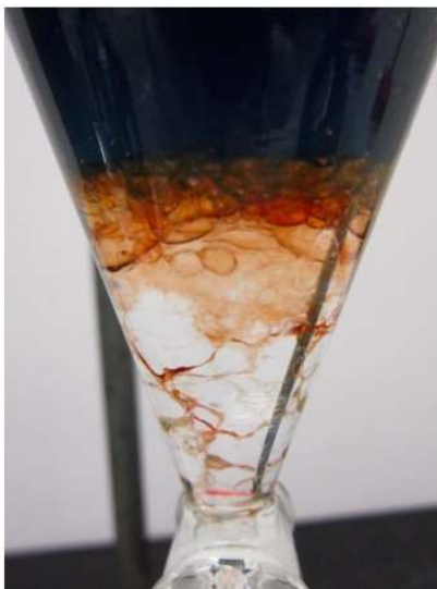
Emulsion formed between dichloromethane and brine (with food coloring).
