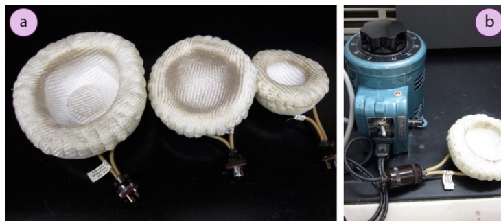
a) Three sizes of heating mantle, b) Heating mantle connected to a Variac.
