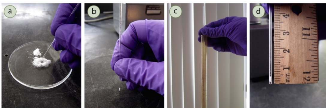
a) Depositing sample into the open end of a capillary tube, b) Inverting and tapping the tube on the benchtop, c) Dropping the sample through a long tube, d) Correct height of sample in the tube
