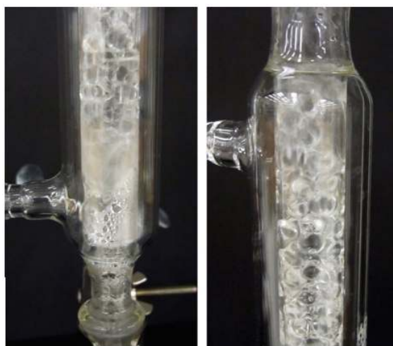
Flooding of a fractionating column
