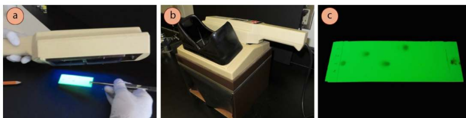
a) Tilting a UV lamp to visualize a TLC plate, b) Box to protect eyes from UV damage, c) Appearance under UV.
