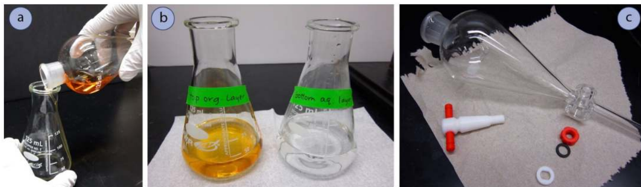
a) Pouring out the top layer, b) Labeled layers, c) Drying the separatory funnel with a disassembled stopcock
