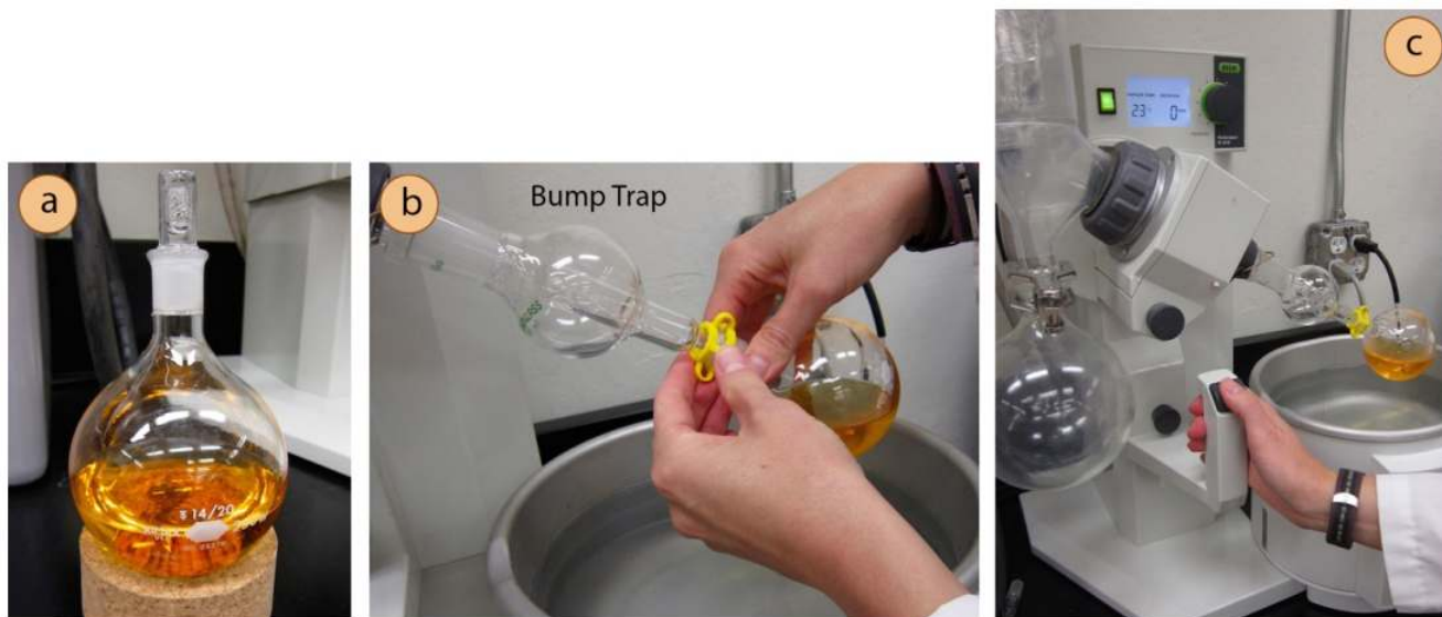
a) Sample to be evaporated, b) Attachment of sample to bump trap on rotary evaporator, c) Lowering of sample into water bath.
