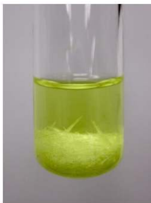
Yellow solid (benzil) in contact with cold ethanol
