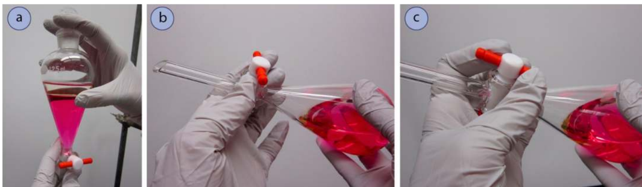
a) Holding the separatory funnel before shaking, b) Inverting the funnel to mix the components, c) Venting to release pressure.
