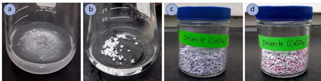
a) Ethyl acetate solution containing fine particles of anhydrous \text{MgSO}_4 , b) Ethyl acetate with clumpy \text{MgSO}_4 hydrate, c) Dry Drierite (blue), d) Wet Drierite (pink)
