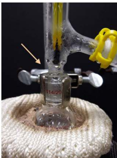
Active distillation. Arrow indicates the joint that needs to be secure to prevent fire.
