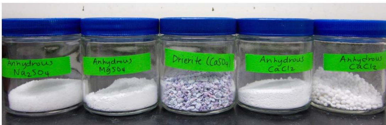
Various drying agents: Anhydrous \text{Na}_2\text{SO}_4 , anhydrous \text{MgSO}_4 , Drierite \text{CaSO}_4 , and anhydrous \text{CaCl}_2 .
