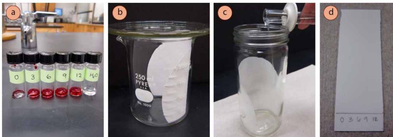
a) Prepared samples, b) TLC chamber made with a beaker and watch glass, c) Adding eluent to a TLC chamber, d) Prepared plate.
