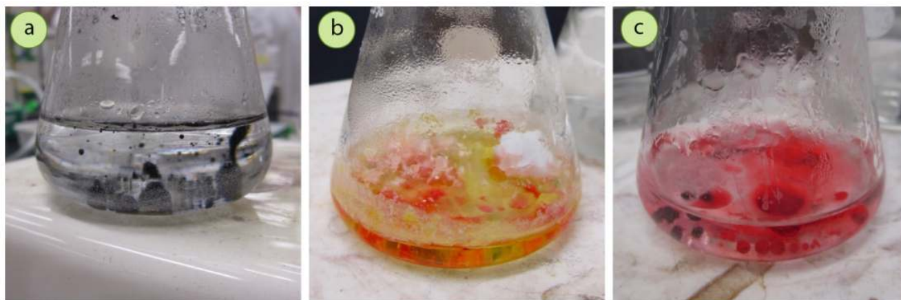
Examples of samples "oiling out" during dissolving: a) Oily droplets of acetanilide in a solution decolorized with charcoal, b+c) Oily droplets containing methyl red and acetanilide in water
