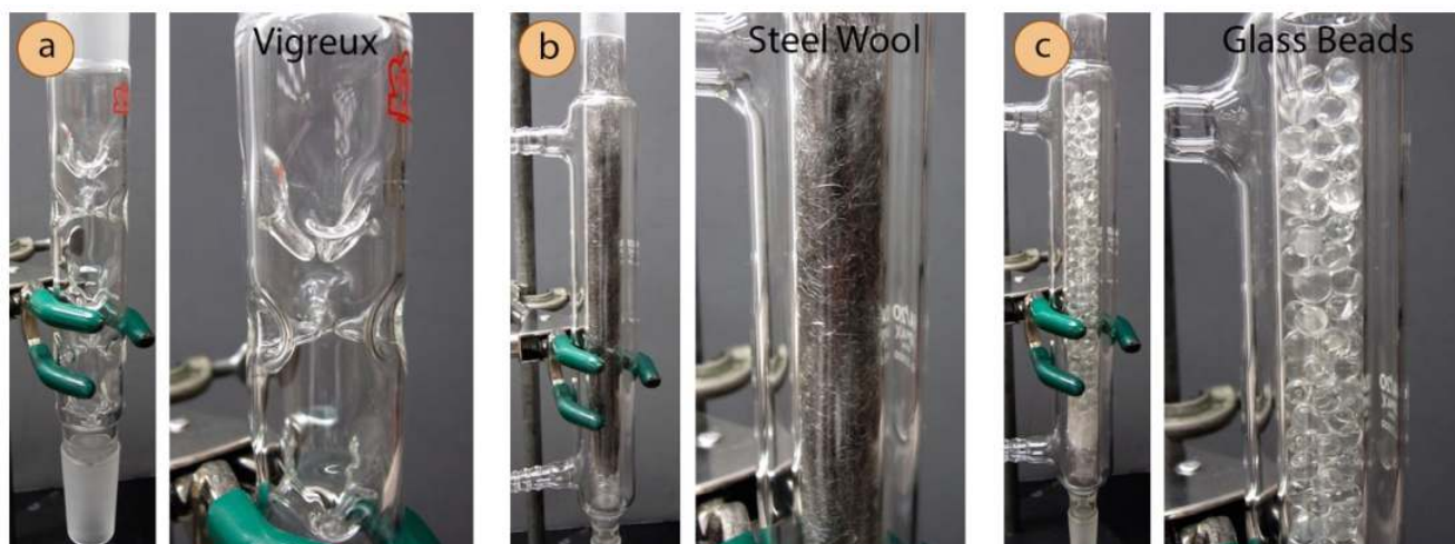
Different fractionating columns: a) Vigreux, b) Steel wool, c) Glass beads
