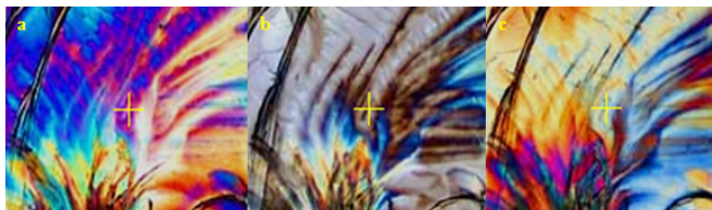
Figure 7.9.11 Cross polarized Microscope images of ascorbic acid specimen with polarizer rotation of (a) 0^\circ , (b) 45^\circ , and (c) 90^\circ . Copyright: Nikon Corporation.
