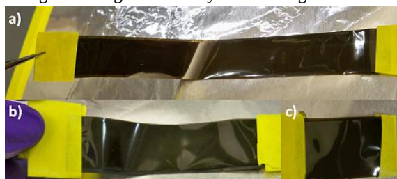
Figure 1.8.16: Folding of the thin film simple once results in a two layer film (a) and after a second and third folding four and eight layers films are obtained (b and c, respectively).
