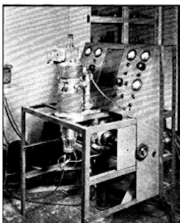
Figure 8.2.19 The first instrument capable of performing electron energy loss spectroscopy built by Hillier and Baker in 1944. Reproduced from J. Hillier and R. F. Baker, J. Appl. Phys. , 1944, 15, 663–675. Copyright AIP Publishing LLC
