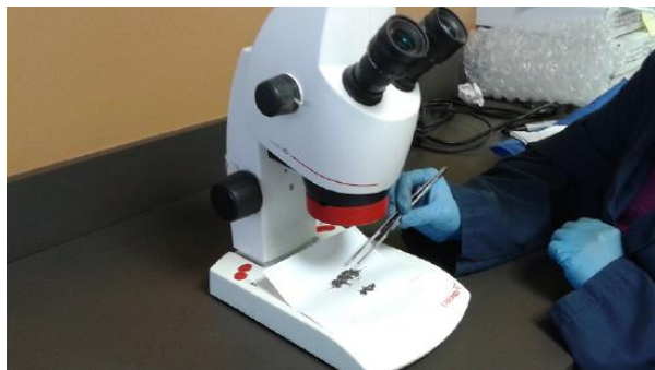
Figure 2.11.6 A light microscope being used to 'pick' the sample. The sample is being separated according to the dominant lithology in preparation for chemical analysis.
