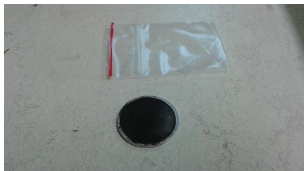
Figure 2.11.9 A completed pellet after pressing.
