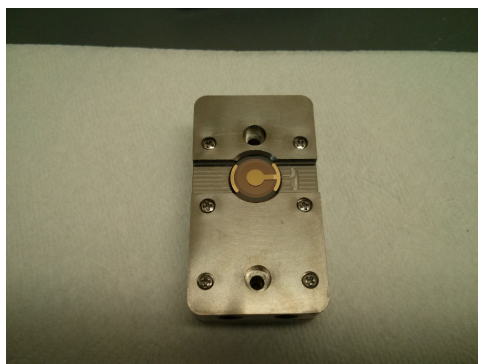
Figure 9.5.4 Correct position of the sensor in the chamber.
