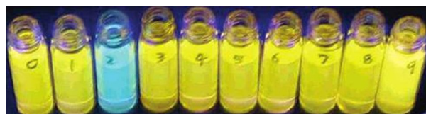
Figure 1.11.11 Fluorescence response of 10 \mu\text{M} RMS in the presence of 20 equiv of different cations of interest at the same condition: control (0), \text{Cd}^{2+} (1), \text{Hg}^{2+} (2), \text{Fe}^{3+} (3), \text{Zn}^{2+} (4), \text{Ag}^+ (5), \text{Co}^{2+} (6), \text{Cu}^{2+} (7), \text{Ni}^{2+} (8), and \text{Pb}^{2+} (9).
