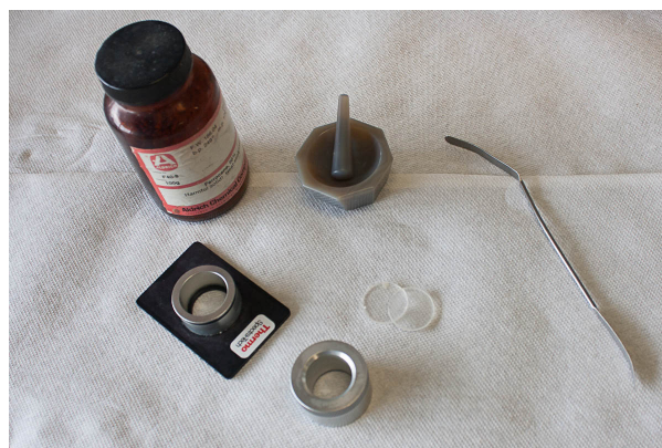
Figure 4.2.2 In this photograph, the sample, ferrocene, two clean and polished KBr plates, an agate mortar and pestle, a mounting card and a spatula are displayed as the base minimum requirements for preparing a sample though a Nujol mull. Of course, a small bottle of mineral oil is also necessary.
