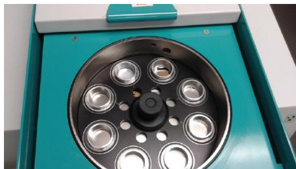
Figure 2.11.11 The inside of the spectrometer where the sample pellets are placed for analysis
