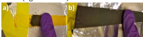
Figure 1.8.14: Making a thin film with a solid sample by (a) dispersing the solid along the Kapton tape and (b) repeated sliding several times to obtain a homogeneous film.
