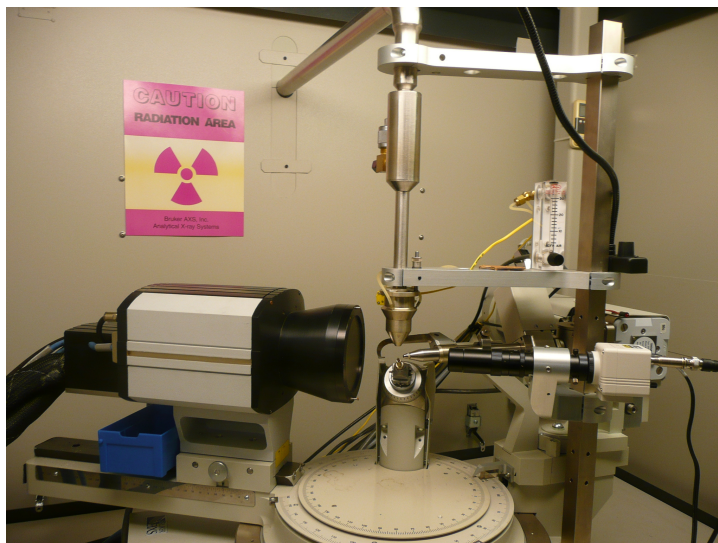
Figure 7.3.9 Single crystal X-ray diffractometer with a CCD detector. The incident beam is generated and delivered through the silver apparatus on the right side of the sample, and the detector is the large black camera to the left of the sample.
