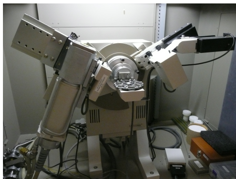
Figure 7.3.16 A powder X-ray diffractometer. Two arms containing the X-ray source and detector are positioned around sample dishes, where the angle between each arm and the plane of the sample dishes is \theta .
