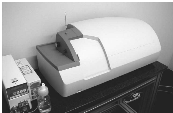
Figure 9.1.11 Picture of the DPI instrument used by Freeman and Cross.
