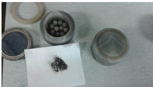
Figure 2.11.3 A milling cup with mill stones and the crushed sample before milling.
