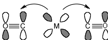
Figure 4.2.22 Schematic representation of competitive back-donation from a transition metal to multiple \pi -acceptor ligands
