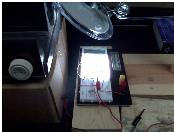
Figure 10.1.6 The picture shows the relative brightness of the light beam at an approximate intensity of 1000 \text{ W/m}^2 . A small concave mirror serves to both turn the beam and to concentrate it a small amount to reach that level.
