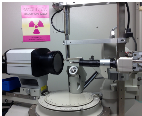
Figure 7.3.28 Modern single-crystal X-ray diffraction machine; the X-ray source can be seen at the right edge as the gray box that extends into the background. Note that the goniometer that holds the crystal in place is not shown.
