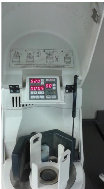
Figure 2.11.2 A Pulsette micro mill, milling cup removed. The mill is set to 520 rotations per minute and a five minute run time.
