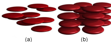
Figure 7.9.3 Schematic representations of (a) a discotic nematic LC phase and (b) a discotic columnar LC phase.
