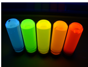
Figure 8.5.12 Fluorescing CdSe quantum dots synthesized in a heat transfer liquid of different sizes (M. S. Wong, Rice University).
