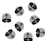
Figure 4.7.46 Representation of nuclei in absence of magnetic field.
