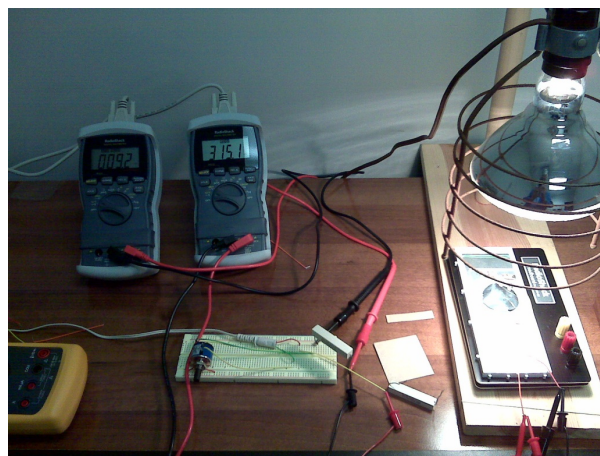
Figure 10.1.2 Simple test apparatus for qualitative measurement of the current-voltage output from an experimental thin film solar cell.
