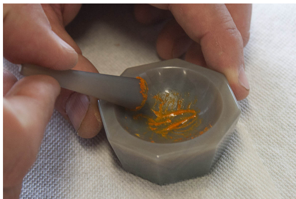
Figure 4.2.3 Mulling ferrocene into mineral oil with a mortar and pestle.
