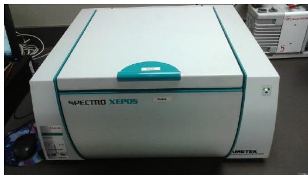
Figure 2.11.10 A Spectro XEPOS X-Ray fluorescence spectrometer.
