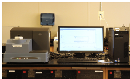
Figure 2.8.26 Picture of basic DSC setup in a laboratory.
