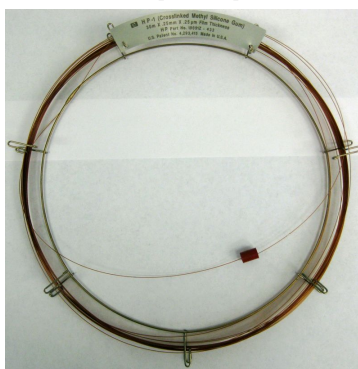
Figure 5.1.3 An example of a capillary column.
