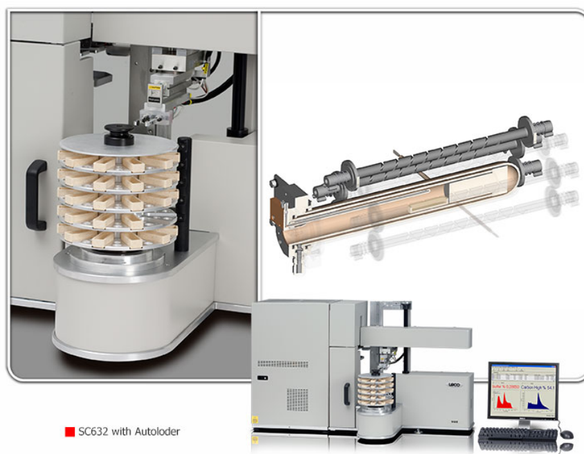
Figure 1.10.2: Example of a LECO analyzer. Samples placed in small cream colored trays and combusted in oven under oxygen atmosphere (big box lower right) computer output to show carbon content. Material used with permission by LECO Corporation
