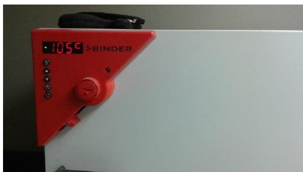
Figure 2.11.5 A drying oven with temperature set above the temperature of evaporation for water at 105 °C
