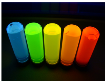
Figure 8.5.44 A picture of different-sized CdSe quantum dots synthesized in a heat transfer liquid (M.S. Wong, Rice University).
