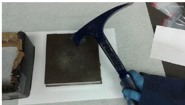
Figure 2.11.1 A hammer and hard surface for crushing. The makeshift cardboard shield on the left can be placed around the hard surface to control fragmentation.
