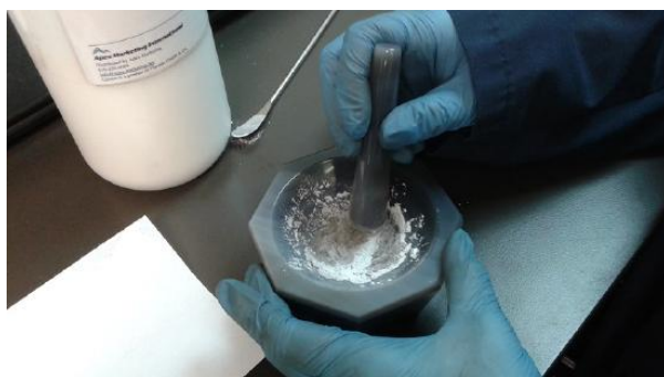
Figure 2.11.7 A mortar and pestle being used to grind the sample to a powder for pelleting in the pellet press. A binding agent (Cereox) is also added using the scapula.
