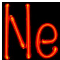
Figure 1.5.1 A Gas Discharge Tube Producing Cathode Rays When a high voltage is applied to a gas contained at low pressure in a gas discharge tube, electricity flows through the gas, and energy is emitted in the form of light. Neon signs work this way
