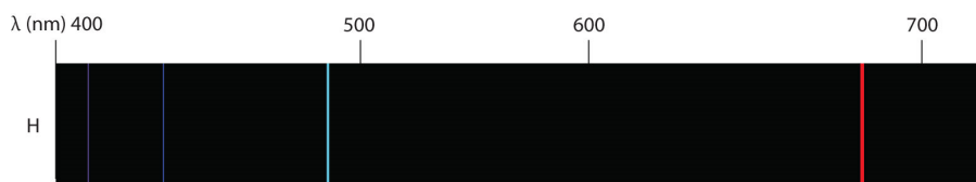
Figure 8.3.2: Hydrogen Spectrum. The spectrum of hydrogen was particularly simple and could be predicted by a simple mathematical expression.
