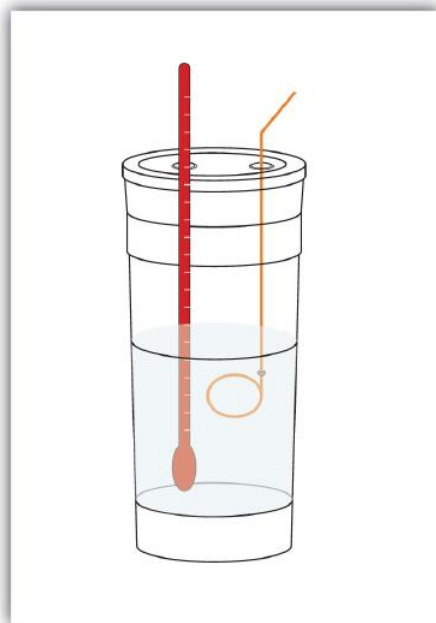
Figure 7.4.2 Calorimeters. A simple calorimeter can be constructed from some nested foam coffee cups, a cover, a thermometer, and a stirrer.
