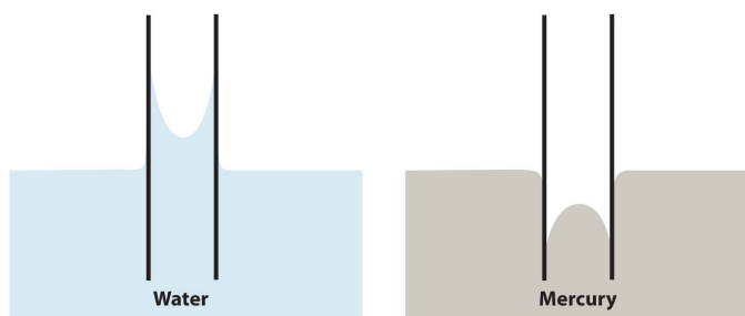
Figure 10.4.7: Capillary Action. (a) Capillary rise is seen when adhesion is strong, such as with water in a thin glass tube. (b) Capillary depression is seen when cohesive forces are stronger than adhesive forces, such as with mercury and thin glass tubes.
