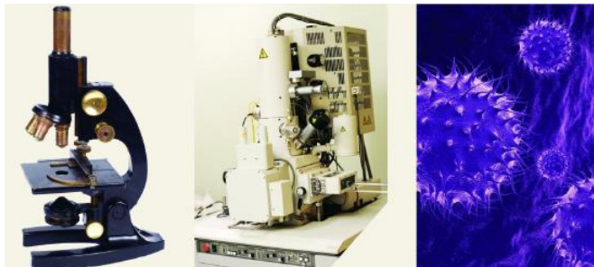
Figure 8.1.1 Microscopes © Thinkstock (a) A simple light microscope can magnify up to 1,500 times. (b) An electron microscope can magnify up to 1,000,000 times. (c) Flu viruses imaged by an electron microscope. The virus is about 100 nm in diameter.
