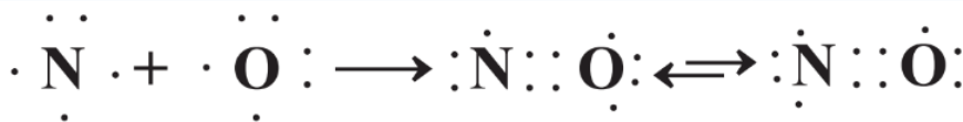
Figure 4.10. Formation of NO. The uneven number of electrons cannot accommodate complete octets around both atoms simultaneously, so the structure is a hybrid resonance structure of the two forms shown.
