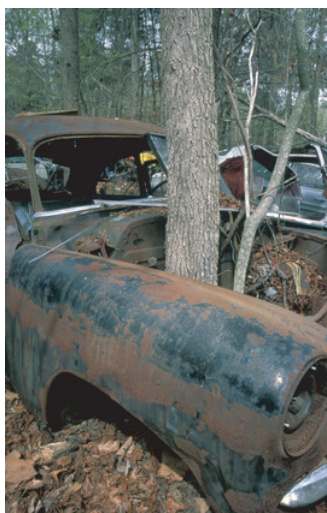
Figure 4.5.2: Rust Formation. The corrosion process involves an oxidation–reduction reaction in which metallic iron is converted to \text{Fe}(\text{OH})_3 , a reddish-brown solid.
