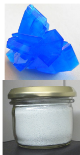
Figure 2.7.1: Loss of Water from a Hydrate with Heating. (left) When blue \text{CuSO}_4 \cdot 5\text{H}_2\text{O} is heated, two molecules of water are lost at 30^\circ\text{C} , two more at 110^\circ\text{C} , and the last at 250^\circ\text{C} to give white "anhydrous" \text{CuSO}_4 (right). Images used with permission from Wikipedia.
