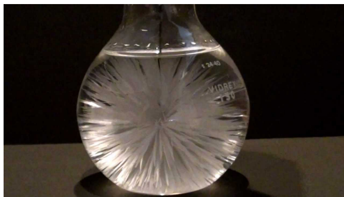
Figure 1.1.4: The Crystallization of Sodium Acetate from a Concentrated Solution of Sodium Acetate in Water. The addition of a small “seed” crystal (a) causes the compound to form white crystals, which grow and eventually occupy most of the flask. Video can be found here: www.youtube.com/watch?v=BLq5NibwV5g
