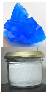
Figure 2.7.1: Loss of Water from a Hydrate with Heating. (left) When blue \text{CuSO}_4 \cdot 5\text{H}_2\text{O} is heated, two molecules of water are lost at 30^\circ\text{C} , two more at 110^\circ\text{C} , and the last at 250^\circ\text{C} to give white "anhydrous" \text{CuSO}_4 (right). Images used with permission from Wikipedia.
