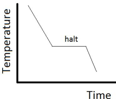
The same data can be obtained by heating the system using a technique such as scanning calorimetry. In this experiment, heat is supplied to a sample at a constant rate, and the temperature of the sample is measured, with breaks occurring at the phase change temperatures.
