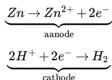
The propensity of zinc to oxidize coupled with that of hydrogen to reduce creates a potential energy difference between the electrodes at which these processes occur. And like any potential energy difference, it can create a force which can be used to do work. In this case, the work is that of pushing electrons through a circuit. The work of such a process can be calculated by integrating
