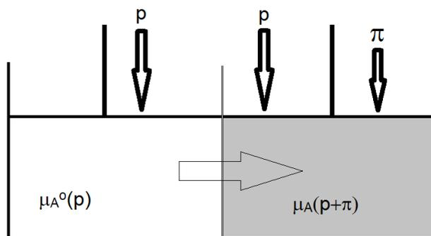
The nature of osmosis and the magnitude of the osmotic pressure can be understood by examining the chemical potential of a pure solvent and that of the solvent in a solution. The chemical potential of the solvent in the solution (before any extra pressure is applied) is given by
