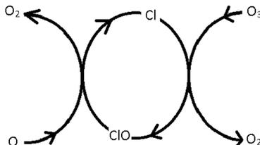
On the left, atomic oxygen picks up an oxygen atom from  $ClO$  to form  $O_2$  and generate a  $Cl$  atom, which can then react with  $O_3$  to form  $ClO$  and an  $O_2$  molecule. The closed loop in the middle is characteristic of the catalytic cycle involving  $Cl$  and  $ClO$ . Further, since  $Cl$  acts as a catalyst, it can decompose many  $O_3$  molecules without being degraded through side reactions.
