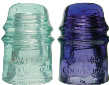
Figure 11.6.1: Radiation Damage. When high-energy particles emitted by radioactive decay interact with matter, they can break bonds or ionize molecules, resulting in changes in physical properties such as ductility or color. The glass electrical insulator on the left has not been exposed to radiation, but the insulator on the right has received intense radiation doses over a long period of time. Radiation damage changed the chemical structure of the glass, causing it to become bright blue.
