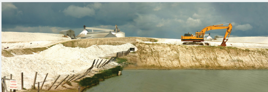
Figure 8.13.5: Salt Mining © Thinkstock. Salt mining can be at the surface or below ground. Here salt is mined from surface deposits. Part of the processing facility can be seen in the background.
