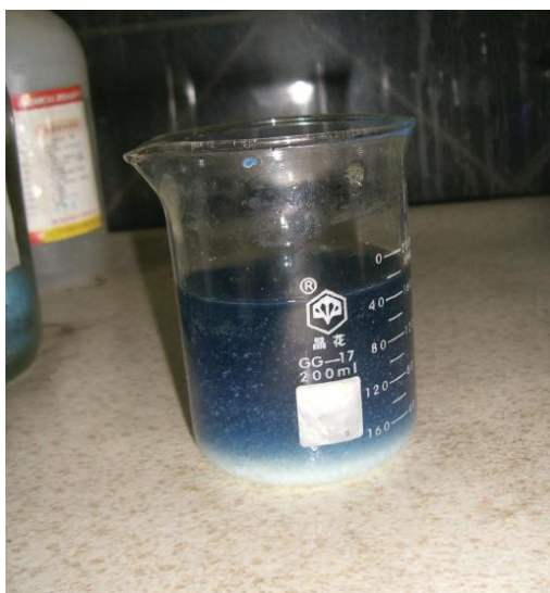
Figure 5.3.2: Double-Replacement Reactions. Some double-replacement reactions are obvious because you can see a solid precipitate coming out of solution. Source: Photo courtesy of Choi, Wikimedia [commons.wikimedia.org].
