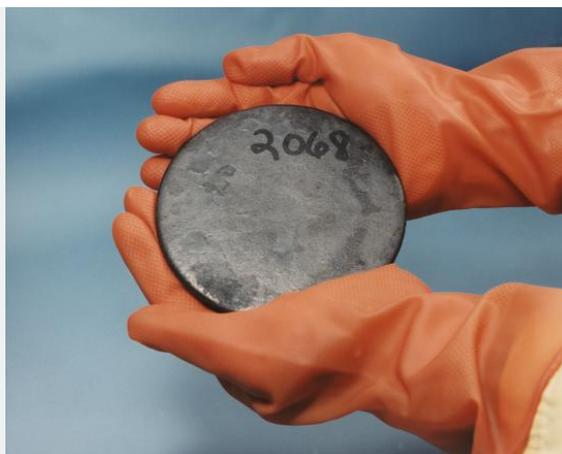
Figure 2.3.3: A billet of highly enriched uranium that was recovered from scrap processed at the Y-12 National Security Complex Plant. Original and unrotated.
