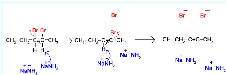
Notice the intermediate of the alkyne synthesis. It is stereospecifically in its anti form. Because the second proton and halogen are pulled off the molecule this is unimportant to the synthesis of alkynes.
