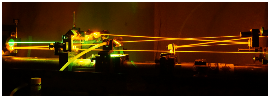
Figure 15.5.3: A dye laser in use. The dye is entering the dye cell through the yellow tube in the left foreground. (CC BY-SA 4.0, By Zaereth - Own work, https://commons.wikimedia.org/w/index.php?curid=55762750 )
