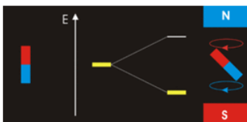
Figure 6.6.3 : The orbiting electron with a non-zero l value acts like a magnetic field with is no energetic difference for any particular orientation (only one energy state, on the left). However, in external magnetic field there is a high-energy state and a low-energy state depending on the relative orientations of the magnet to the external field. (CC SA-BY 3.0; Darekk2).
