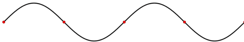
Figure 2.1.4 : Animation of standing wave in the stationary medium with marked wave nodes (red circles). (public domain; LucasVB).
