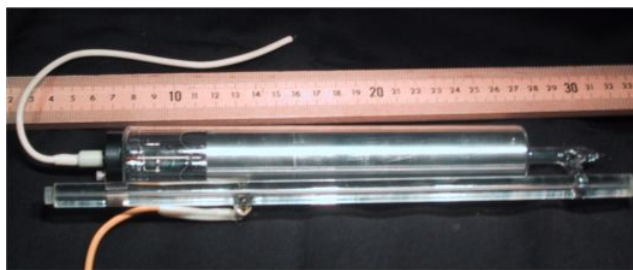
Figure 15.6.3: A commercial He-Ne tube. The thicker cylinder closest to the meter-stick (shown for scale) is the ballast. The thinner tube houses the resonant cavity where the lasing occurs. Notice the two mirrors that seal the two ends of the bore. For mode stability reasons, these mirrors are concave; they serve as the output coupler and the high reflector. (Copyright; author via source)
