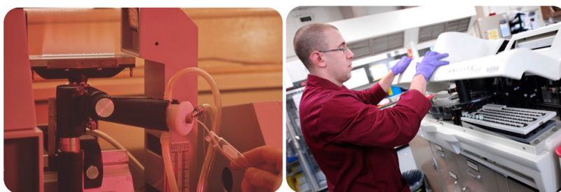
Figure 1.1.2: (left) Measurement of trace metals using atomic spectroscopy. (right) Measurement of hormone concentrations.
