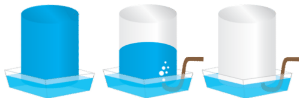
Figure 11.10.2: A gas produced in a chemical reaction can be collected by water displacement.
