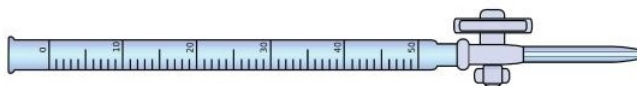
Figure 14.6.1: Equipment for Titrations. A burette is a type of liquid dispensing system that can accurately indicate the volume of liquid dispensed.
