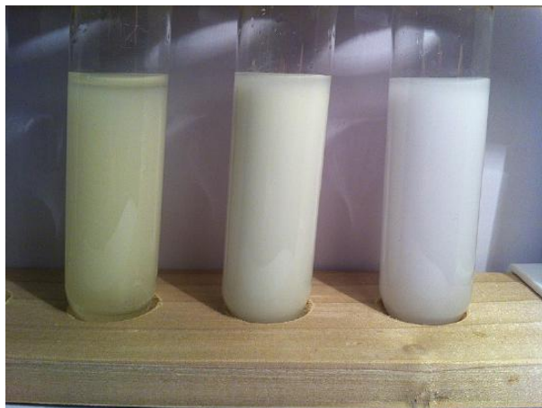
Figure 7.6.1: The three common silver halide precipitates: AgI, AgBr and AgCl (left to right). The silver halides precipitate out of solution, but often form suspensions before settling. (CC BY-SA 3.0; Cychr).
