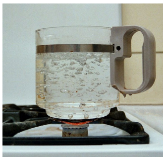
Figure 12.5.1: The Boiling Point of Water. Nucleate boiling of water over a kitchen stove burner. (Source: Wikipedia). Water is a good substance to use as an example because many people are already familiar with it. Other substances have melting points and boiling points as well.
