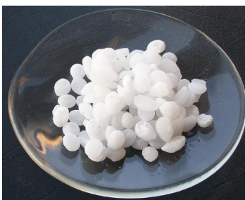
Figure 14.3.1: Sample of sodium hydroxide as pellets in a watch glass. (Public Domain; Walkerma.)
