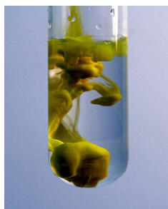
Figure 7.10.3: Lead (II) iodide precipitates when potassium iodide is mixed with lead (II) nitrate (Equation 7.10.1). (CC BY-SA 3.0; PRHaney).
