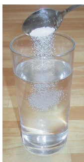
Figure 13.2.1: Making a saline water solution by dissolving table salt (NaCl) in water. The salt is the solute and the water the solvent. (CC-BY-SA 3.0; Chris 73).
