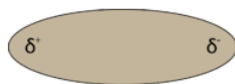
Figure 10.8.6: A dipole is any molecule with a positive end and a negative end, resulting from unequal distribution of electron density throughout the molecule.
