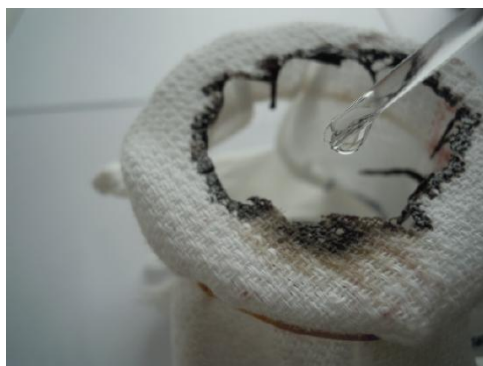
Figure 14.2.1: Drops of concentrated sulfuric acid rapidly decompose a piece of cotton towel by dehydration. (CC BY-SA 3.0; Toxic Walker).
