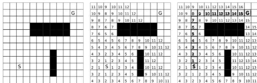
Figure 4.2.3: Dijkstra's algorithm finding a shortest path from 'S' to 'G' assuming the robot can only travel laterally (not diagonally) with cost one per grid cell. Note the few number of cells that remain unexplored once the shortest path (grey) is found, as Dijkstra would always consider a cell with the lowest path cost first.
